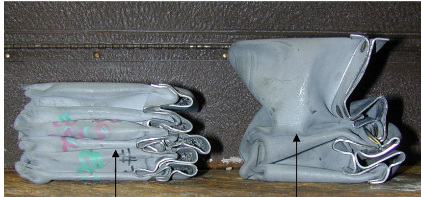
Aluminum Foam Filled Hat Section (after crushing)
