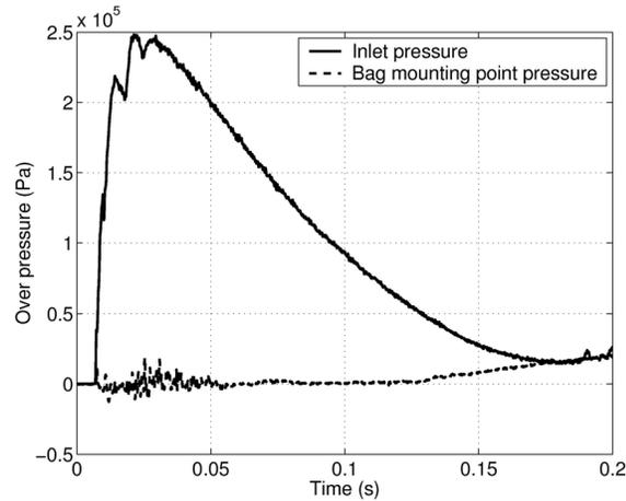
Figure 2. Inlet and bag mounting point pressure
