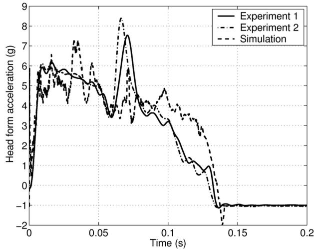
Figure 6. Comparison of Head Form velocity from test and Multi Material ALE simulation
