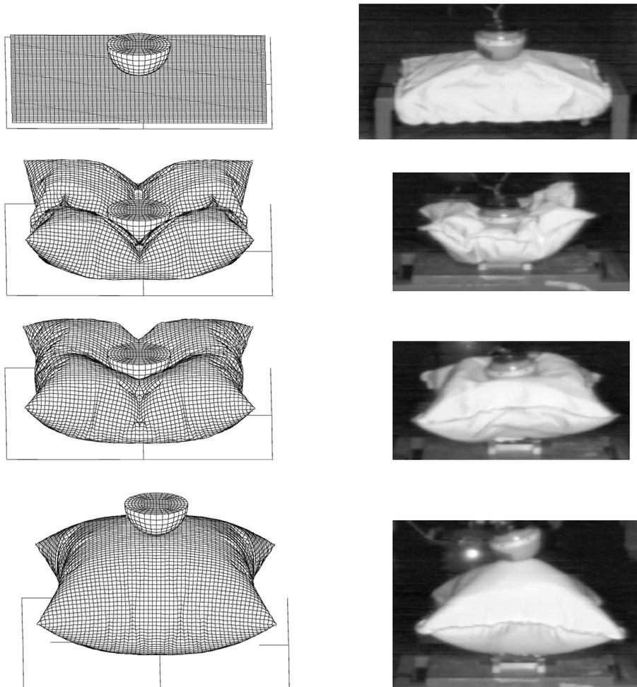
Figure 8. Deformed states from simulation and test at t=0, 40, 80, 120 ms
