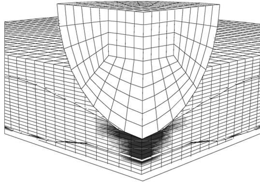
Figure 7. Pressure zone between inlet and Head Form
