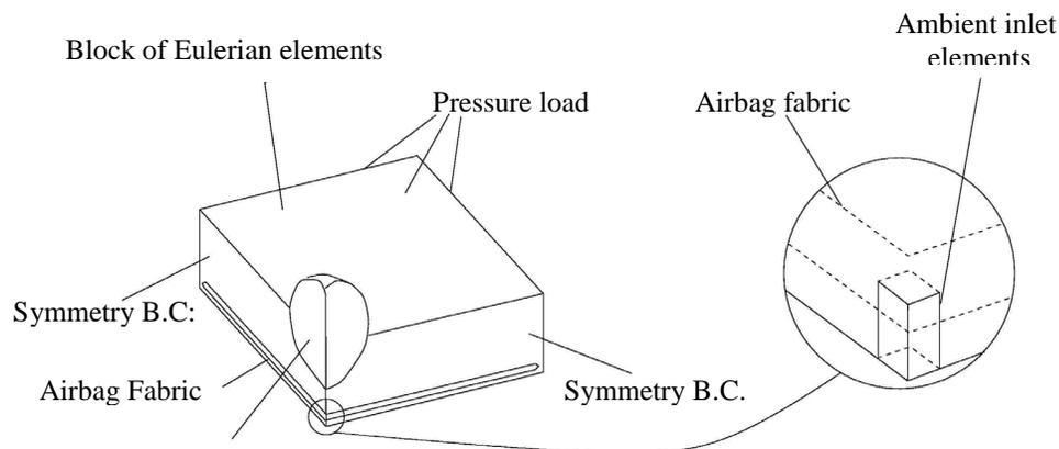
Figure 4. FE-model setup
