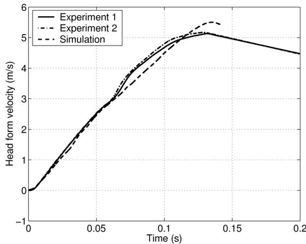
Figure 5. Comparison of Head Form acceleration from test and multi-material ALE simulation
