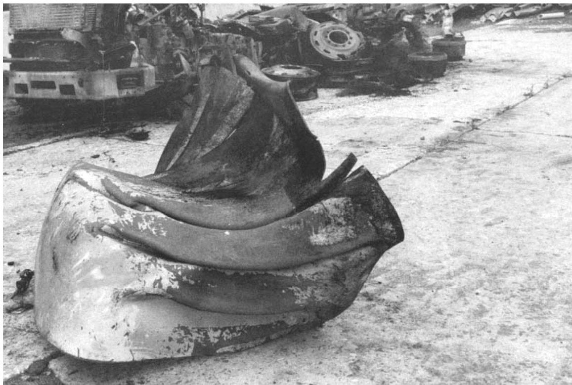
Figure 7. Actual Propane Tank Head
