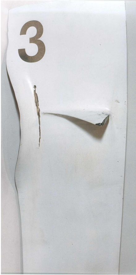
Figure 2. Deformed Blade with Crack
