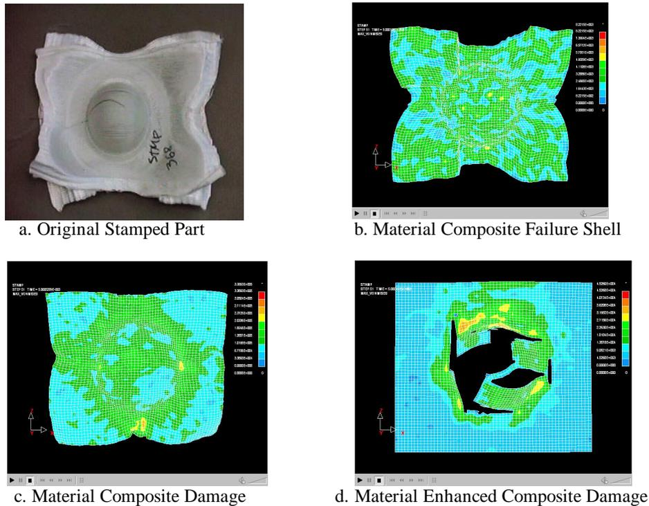
Figure 4. Comparison of Experimental and LS-DYNA Results
