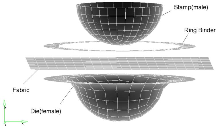
Figure 3. Finite Element Models of Stamping Process Components
