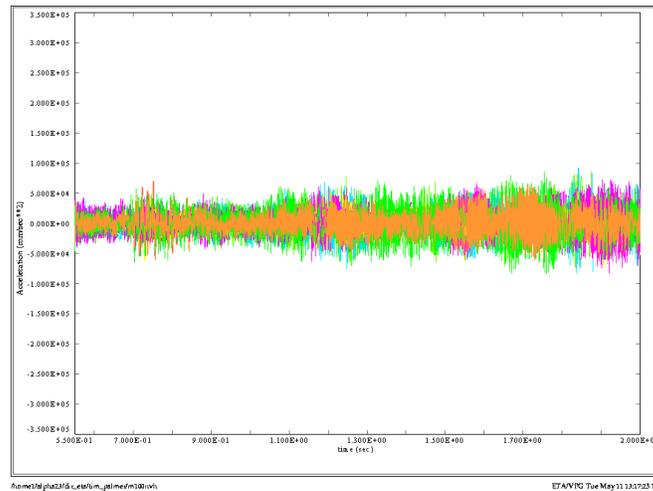
Figure 9: X,Y,Z Acceleration vs. Time for Belgian Block Road
