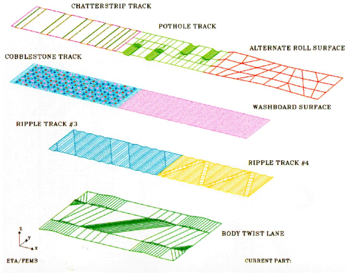
Figure 2. Road Surface Finite Element Models
