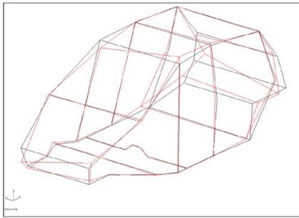
Figure 13: Full Torsion @ 35 Hz
