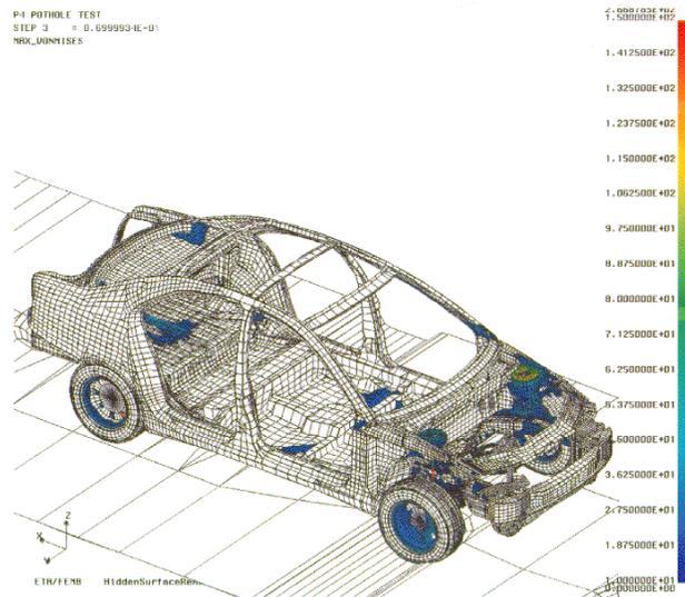
Figure 5. Pothole Track Stress Results at 0.7 seconds
