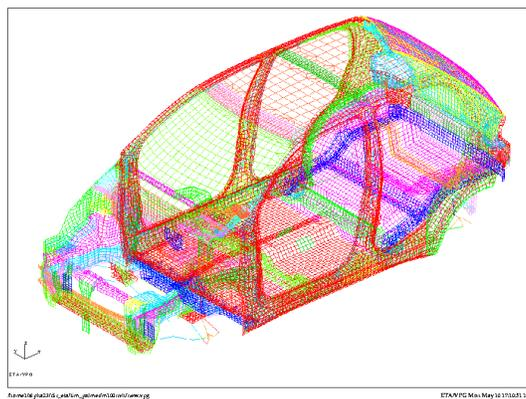
Figure 7: Vehicle Structure and Suspension System for NVH Analysis
