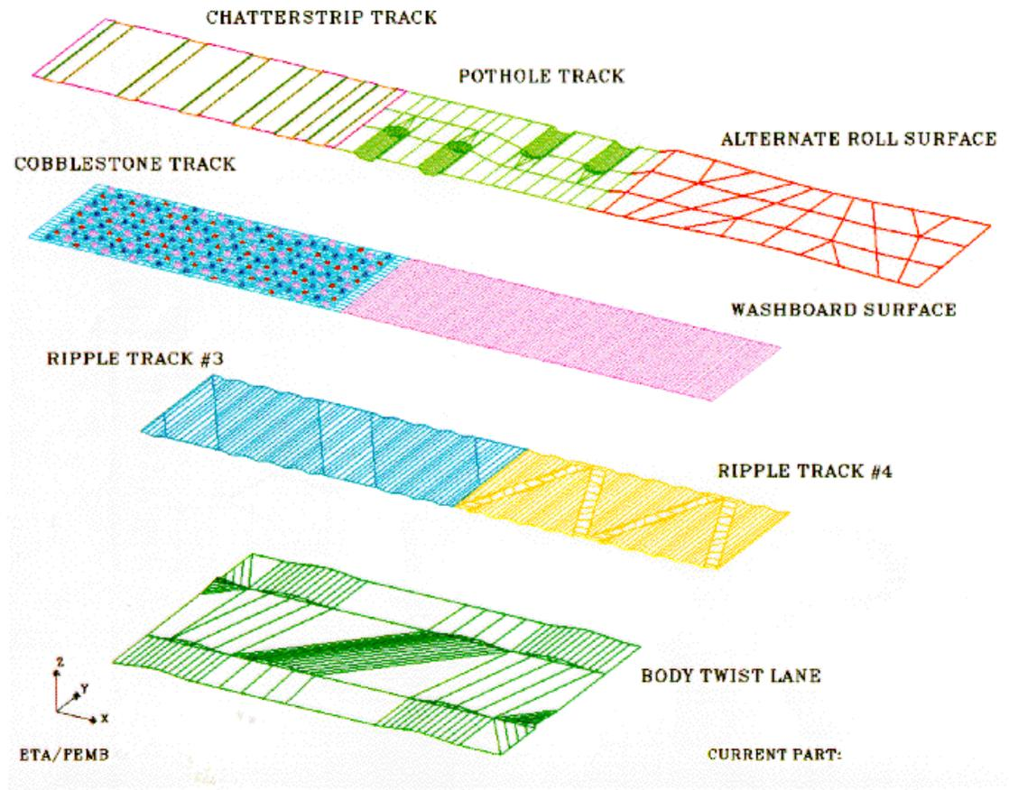
Figure 2. Road Surface Finite Element Models
