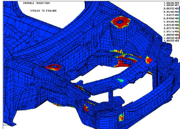
Figure 6: Fatigue Analysis Results for Pothole Condition
