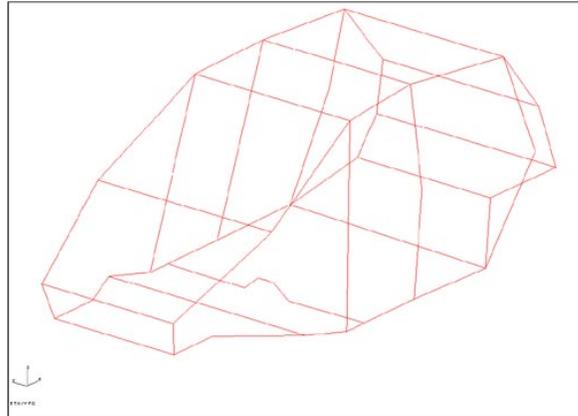
Figure 8: Display Model for NVH Analysis
