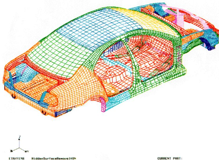
Figure 3. Body-in-White Finite Element Model
