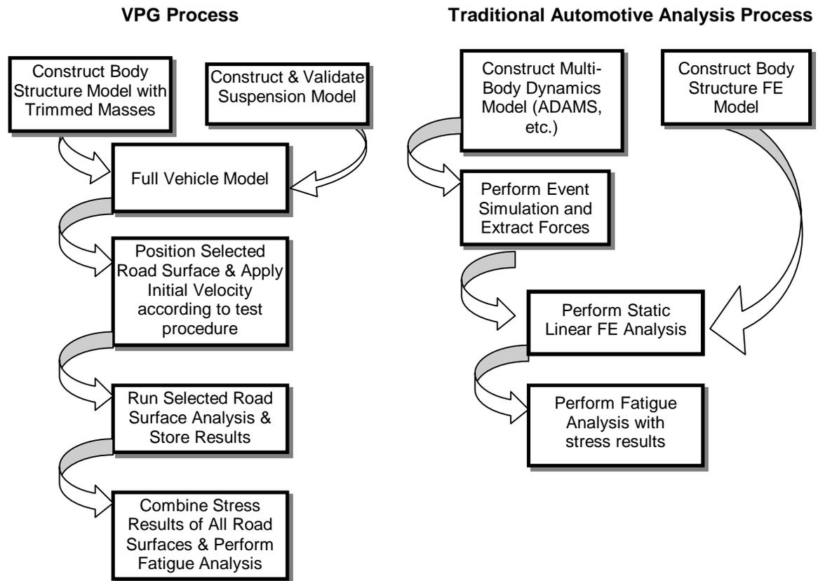
Figure 1. Traditional Automotive Durability Analysis Methodology Process vs. VPG Process
