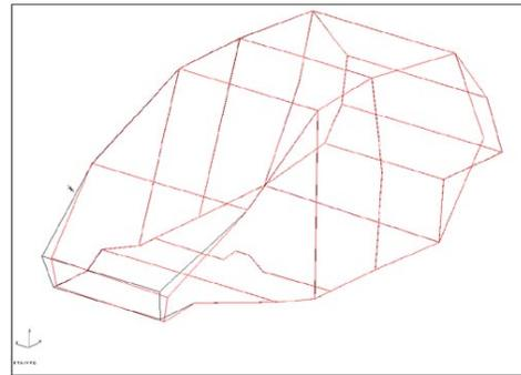
Figure 12: Front End Lateral Bending @ 19Hz
