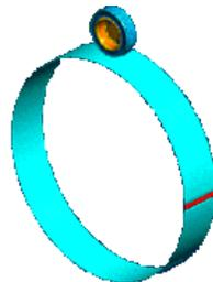
Figure 18. Tire Cleat Test
