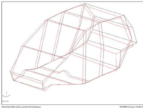
Figure 11: Front Lateral Bending , Vehicle Pitch @ 10.2 Hz
