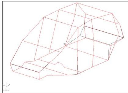
Figure 15: Rear Lateral Bending at 152 Hz.
