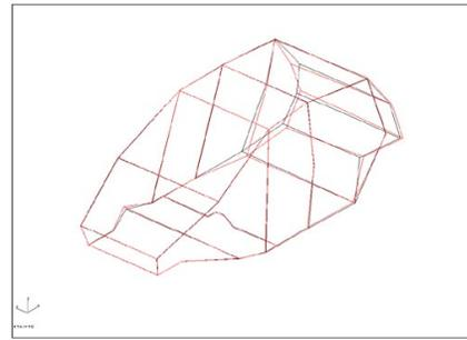
Figure 14: Rear Lateral Bending @ 51 Hz
