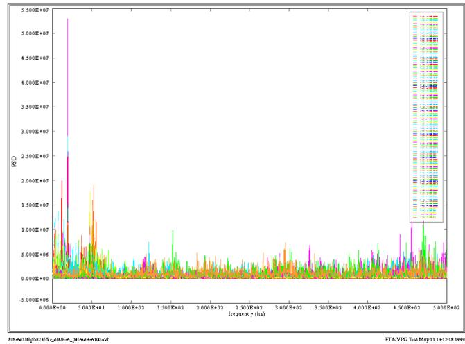
Figure 10: PSD vs. Frequency for Belgian Block Road
