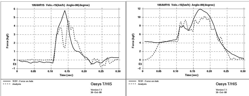
Fig.21 : Longitudinal Axle Force (195 Tire) Fig.22 : Vertical Axle Force (195 Tire)
