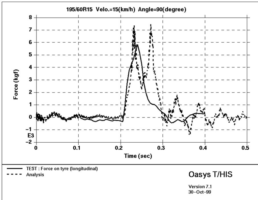
Fig. 26 : Longitudinal Axle Force BiW + FE Tire Model
