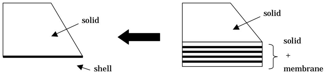
Fig.6 : modeling method of fiber reinforced rubber
