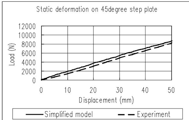
Fig.9 : Static deformation with loading
