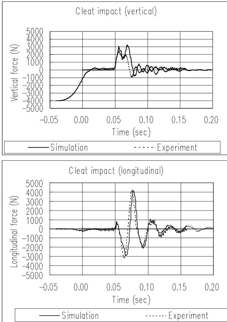
Fig.13 : Cleat impacting force
