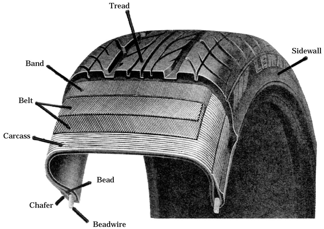
Fig.1 : Tire construction
