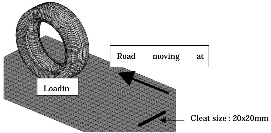
Fig.10 : Boundary condition for cleat impacting simulation
