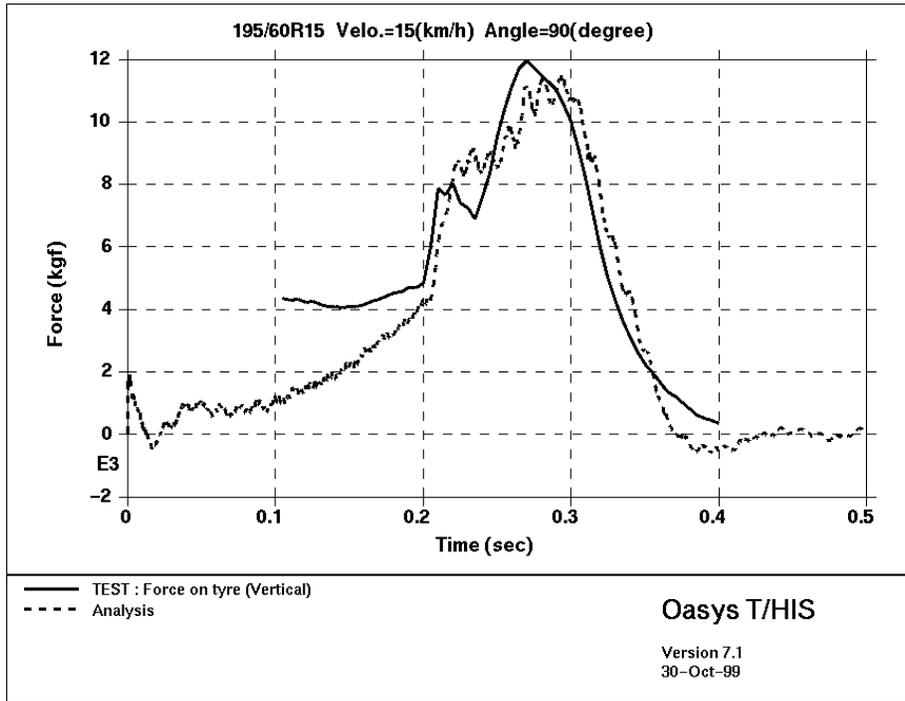
Fig. 25 : Vertical Axle Force BiW + FE Tire Model
