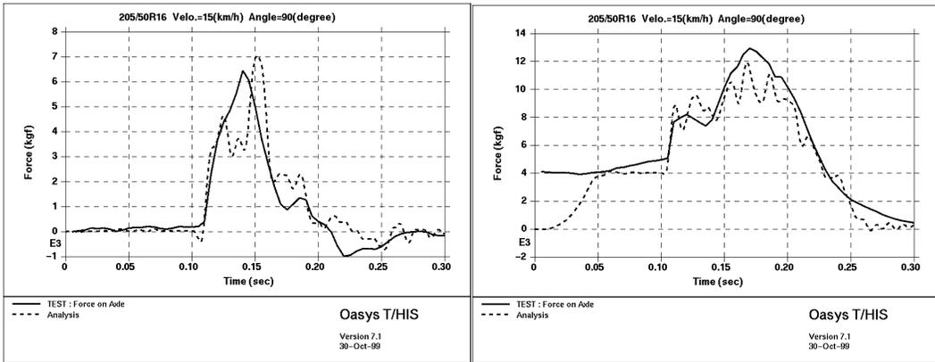
Fig.18 : Longitudinal Axle Force (205 Tire) Fig.19 : Vertical Axle Force (205 Tire)
