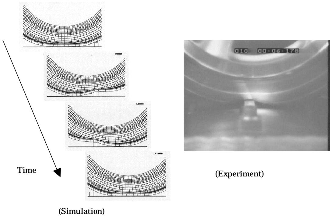
Fig.12 : Cleat impacting shape
