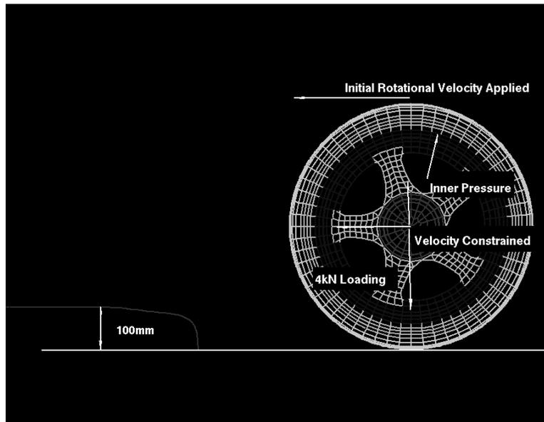
Fig. 16 Curb Strike Model Using Tire Only 205 Tire
