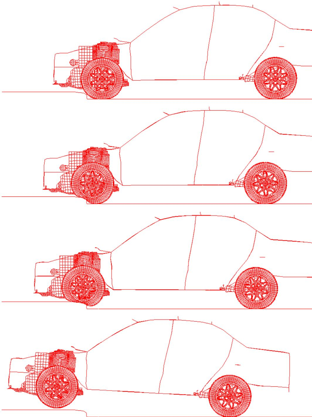
Fig. 24 : Deformation (195 Tire Used)
