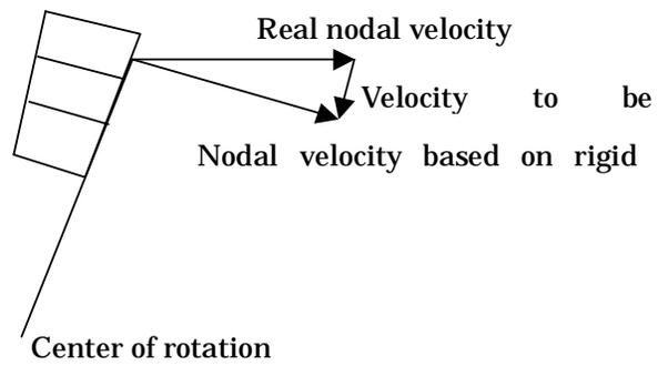
Fig.11 : Method of damping definition
