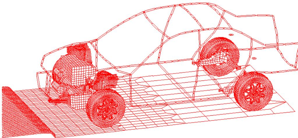
Fig.17 Curb Strike Model With Body + FE Tire 195/60R15 Tire
