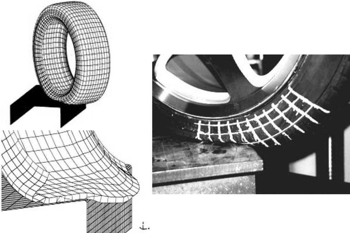
(45 degree step plate : Left : Simulation Right : Experiment)
