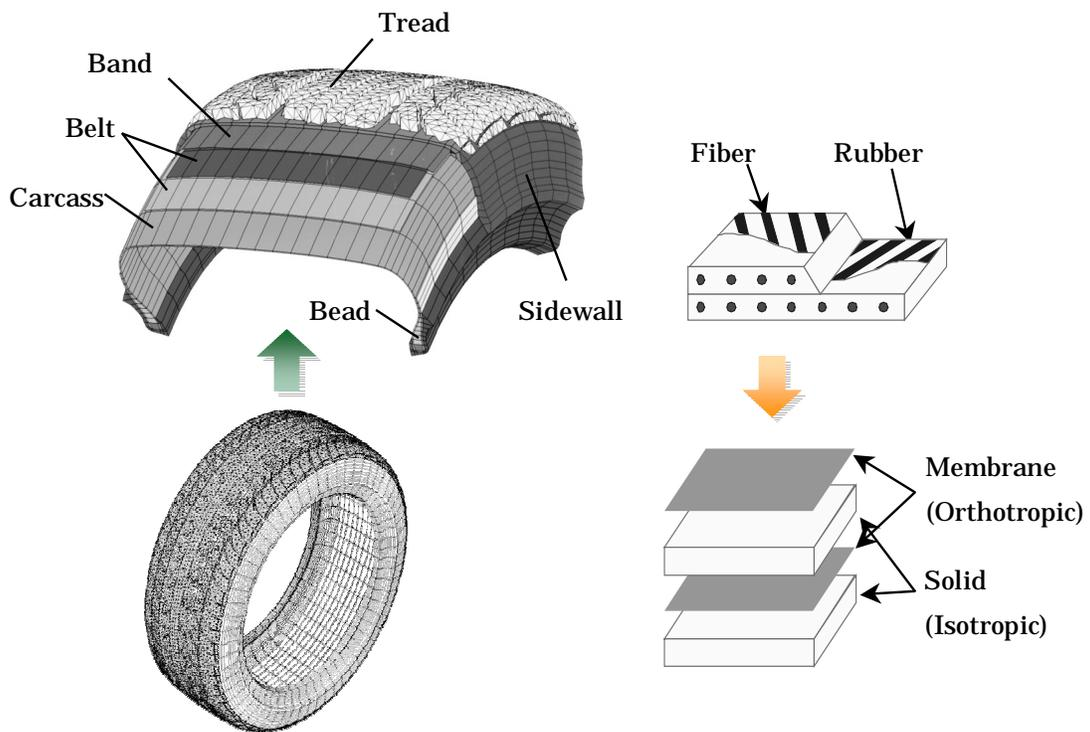
Fig.2 : Tire simulation model
