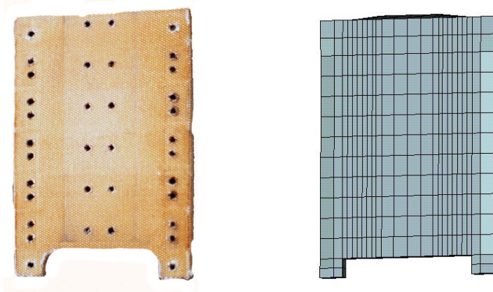
Figure 2: Rib hinge of the USSID, original part and FE model.
