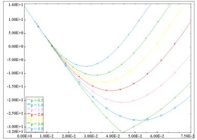
Figure 12. Lander Vertical Coordinate - Various Initial Airbag Pressures
