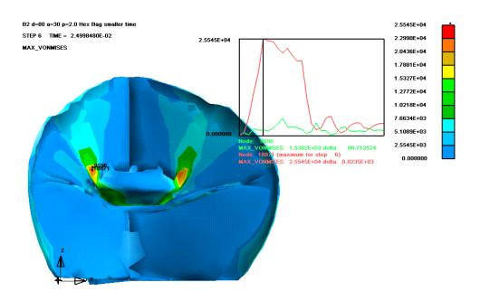
Figure 4. View of Peak Fabric Stress - Face Region of the Airbag
