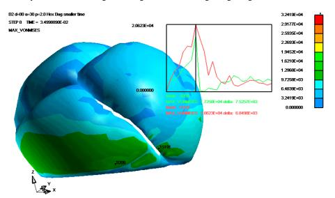
Figure 5 presents the same data plotted on the un-deformed airbag shape. This presentation is particularly useful for defining stress regions to the airbag design engineer.
