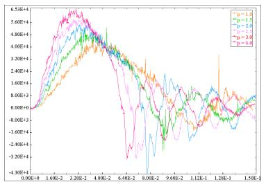
Figure 11. Lander Acceleration Time History - Various Initial Airbag Pressures
