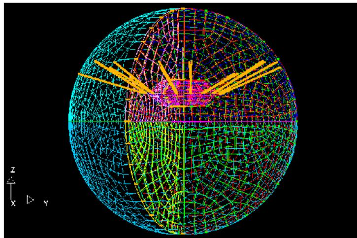
Figure 13. View of Spokes Configuration Added to Model
