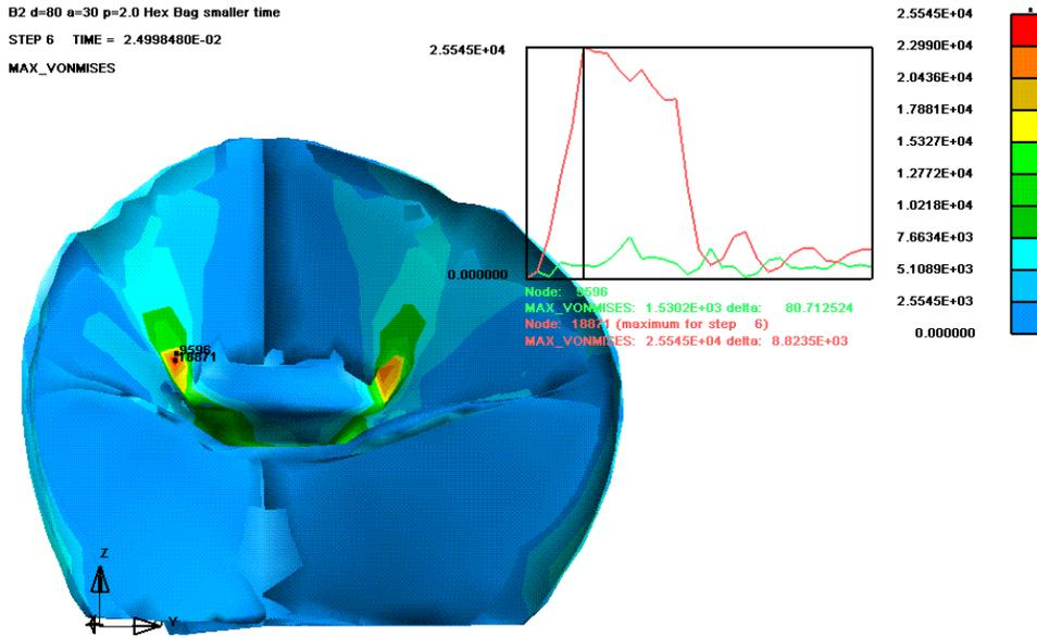
Figure 4. View of Peak Fabric Stress – Face Region of the Airbag
