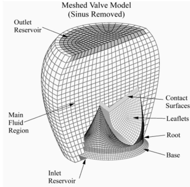
Figure 4. The aortic valve model, showing the inlet and outlet reservoirs. A third reservoir covers the lateral surface, allowing for lateral flow as the sinuses (not shown) and aortic wall expand and contract.
