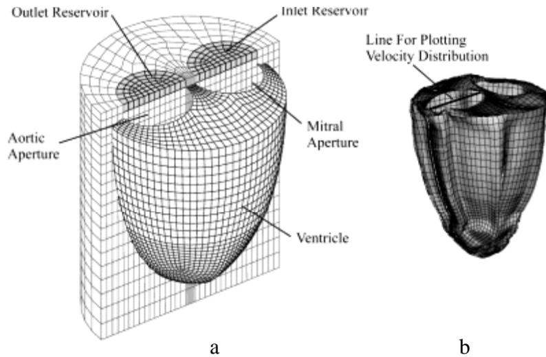
Figure 1. The model of the left ventricle: (a) a section of the fluid control volume revealing the undeformed mesh of the ventricle; (b) the shape of the ventricle after deformation.
