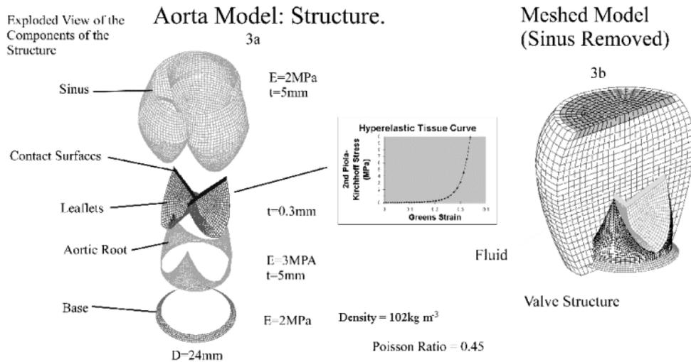
Figure 3. Exploded view of the aortic valve structure showing (a) the dimensions and material properties used, and (b) the leaflets of the valve embedded in the containing fluid control volume.
