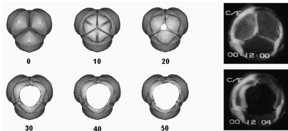
Figure 5. Opening sequence of the model (on the left) in comparison with two images (on the right) from a pulse duplicator study of the opening phase of a bioprosthesis valve.
