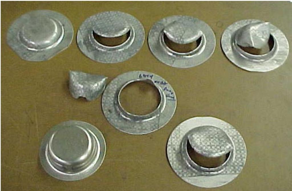
Fig 1: Aluminum cups drawn without any lubricant. Binder force = 6,000 lb approx.
