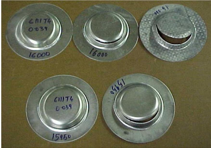
Fig 2: Failure of repeatability tests without any lubrication
