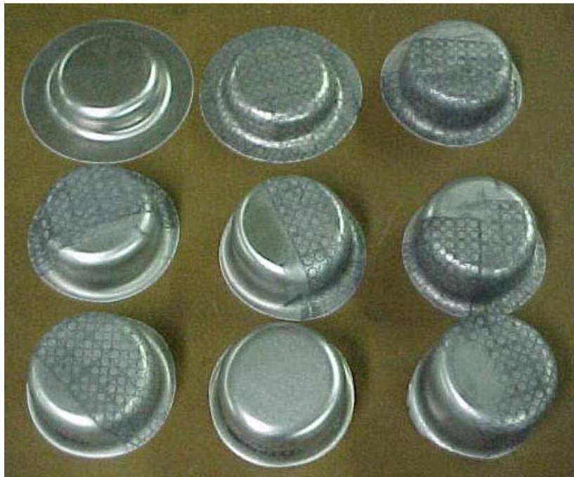
Fig. 3: Successive draws to full depth of the cup with polyurethane paper
