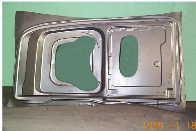
Figure 1. Actual inside rear door on the car
