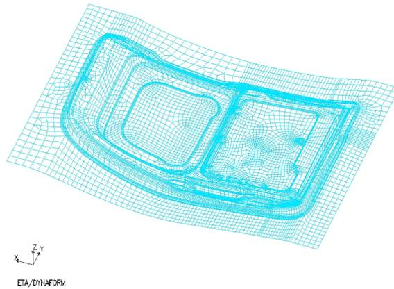
Figure 3. Meshes of inside rear door on the car
