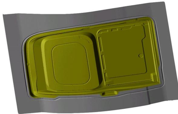
Figure 2. Geometry of inside rear door on the car
