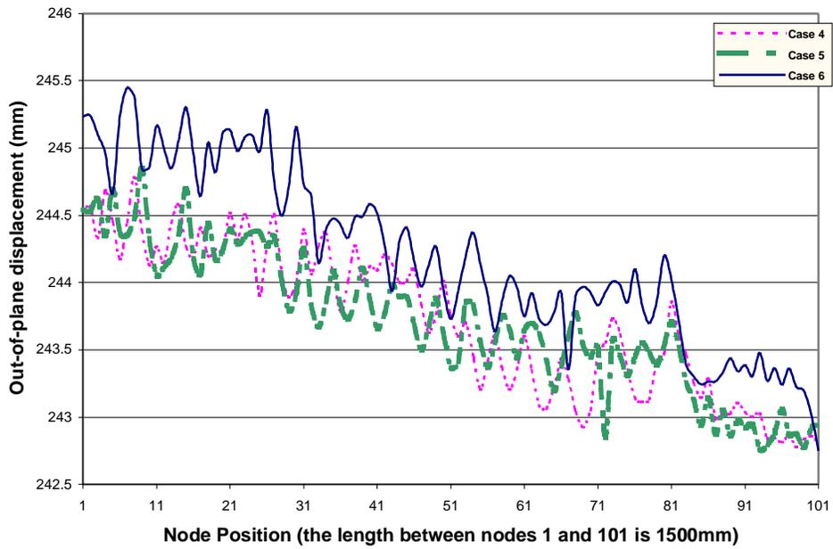
Figure 10. Out of plane displacements from US Steel data (see Table 3).
