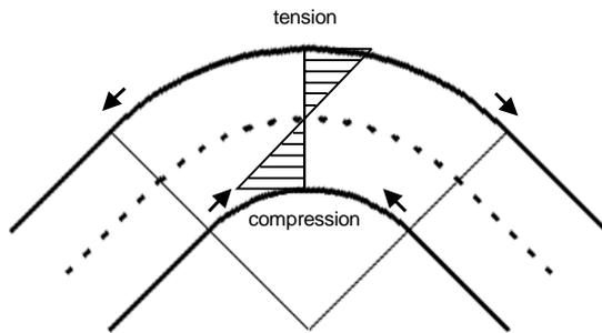
metal (outside of bending lines are strained, and inside of bending lines are compressed as shown in Figure 5). If the material is not stressed over the yield limit, it will spring back. For the large radii, the permanent deformation may not be reached. Therefore, it is very difficult to roll form metals with the bending radius 10 to 100 times (or more) of the material thickness. (Dobrev & Halmos 1997)
