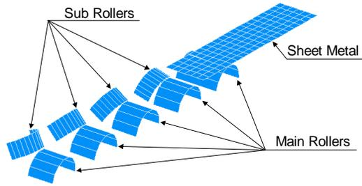
Figure 4. Typical rolling mill setup (upper rollers are not shown for clarity).
