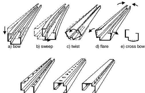
Figure 2. Undesirable effects found in cold roll form sections. (Halmos, 1997)
