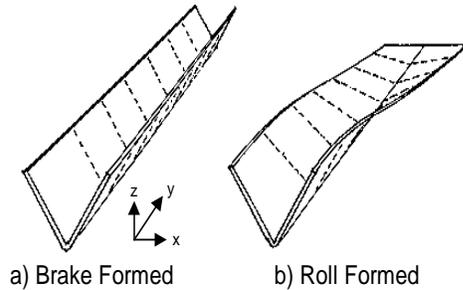
Figure 1. Cross Section Changes in Brake and Roll Formed “V” Section. (Halmos, 1997)
