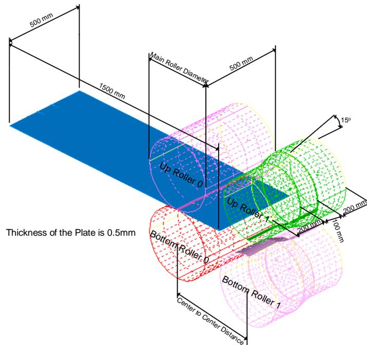
Figure 8. The Model of rolling mill setup.
