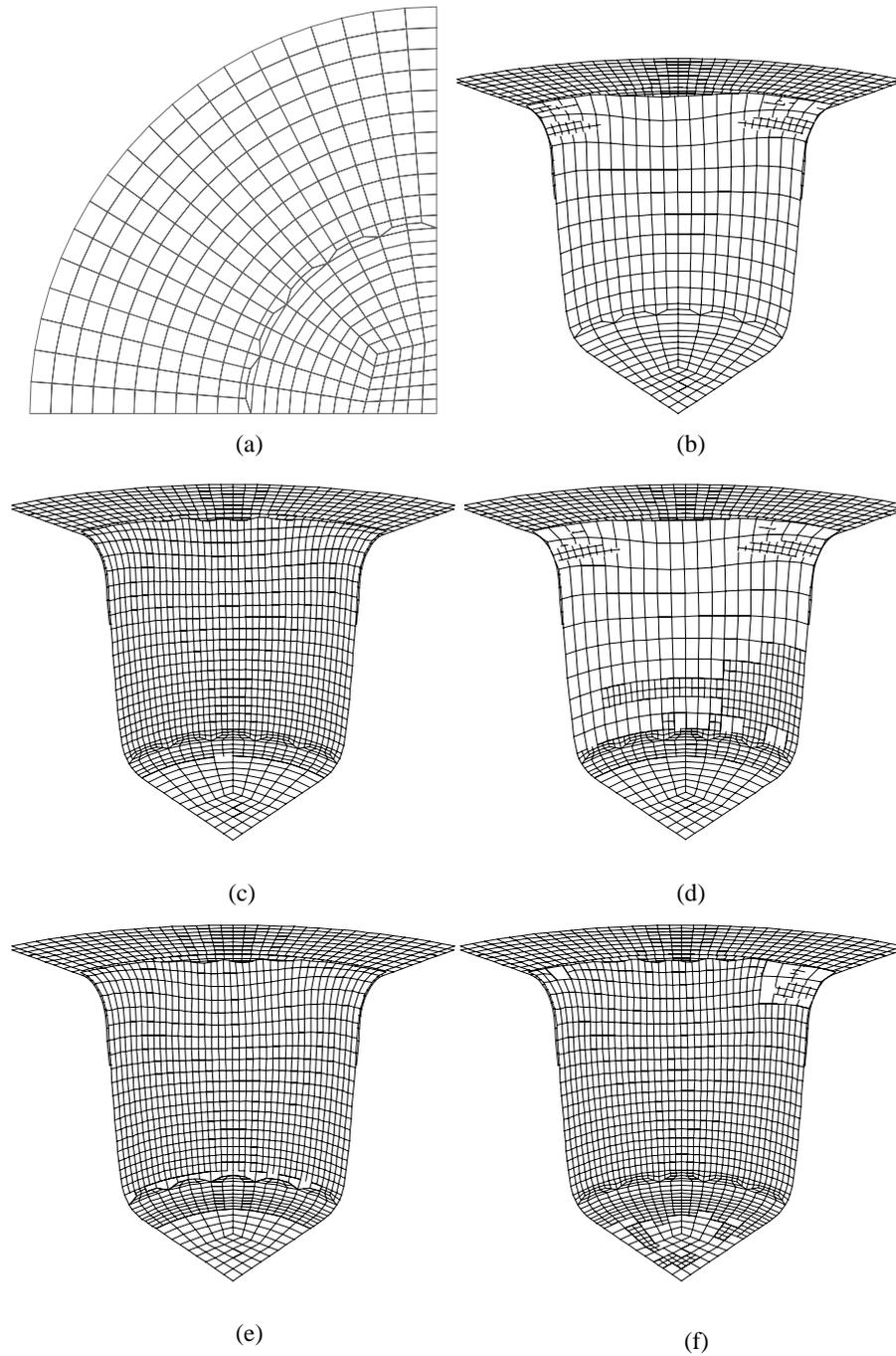
Figure 7. Deep drawing of a cup. (a): Initial geometry of the blank with 335 shell elements. (b): Deformed blank no adaptive mesh refinement. (c): Angle based refinement. (d): Thickness based refinement. (e): GEPS based indicator. (f): GSIG based indicator
