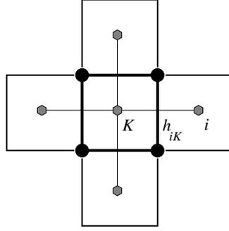
Figure 2. Nodal patch used to compute the refinement indicators
