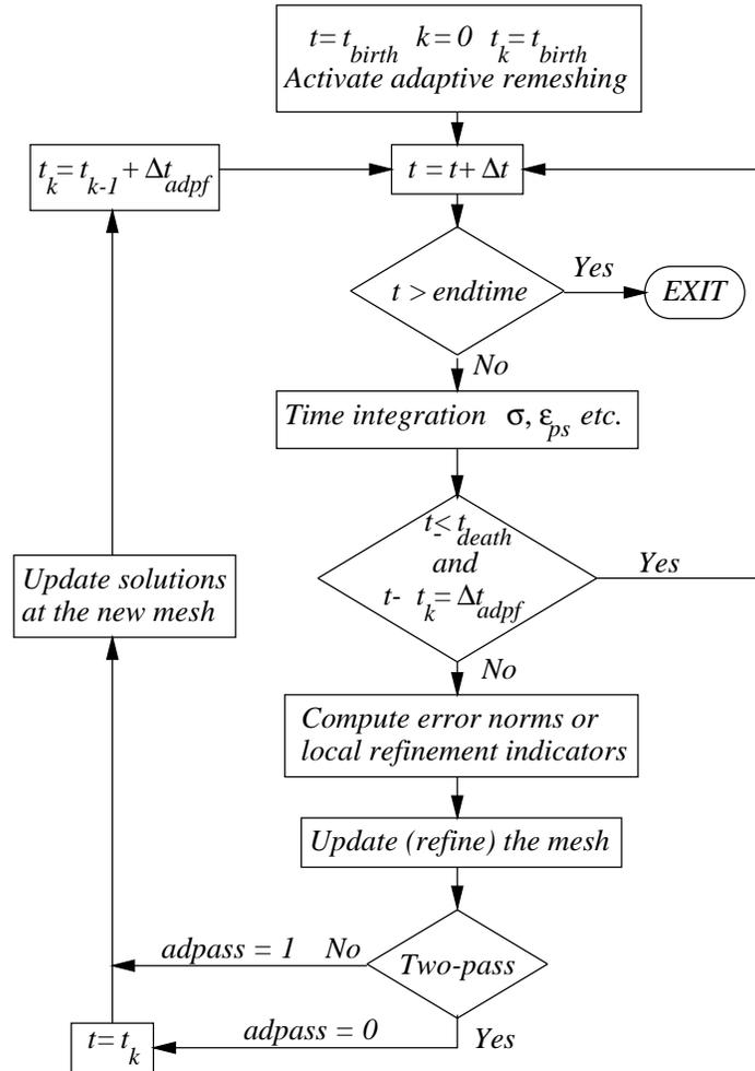
Figure 3. A flowchart illustrating the proposed adaptive procedure
