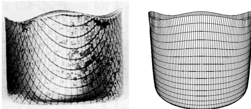
Figure 6. Earing of a drawn cup. Left: Experiment; see (Brännberg 1994). Right: Result from LS-DYNA.
