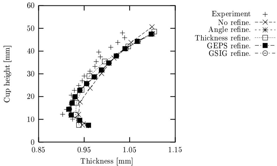
Figure 8. Thickness distribution in the rolling direction
