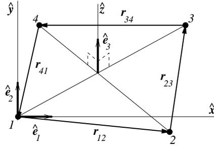
Figure 1. 4-nodes quadrilateral shell element
