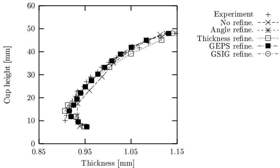
Figure 9. Thickness distribution in 45° to the rolling direction
