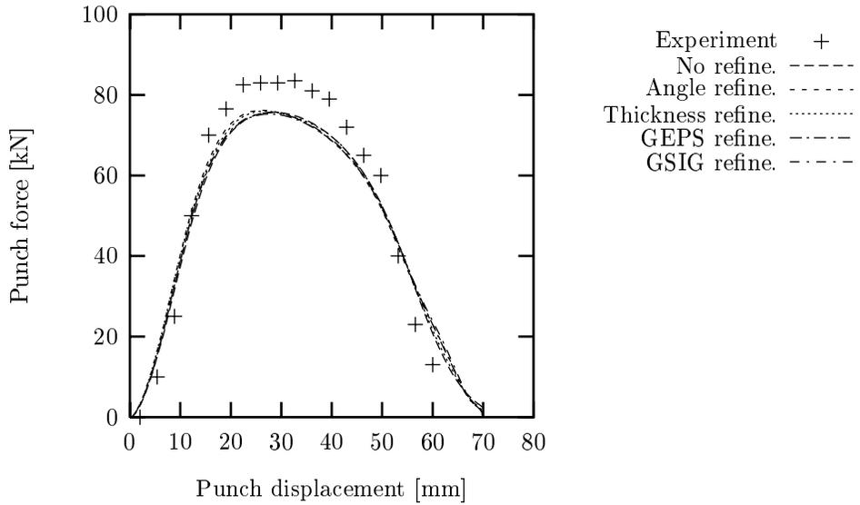
Figure 11. Numerically and experimentally obtained punch force versus punch displacement
