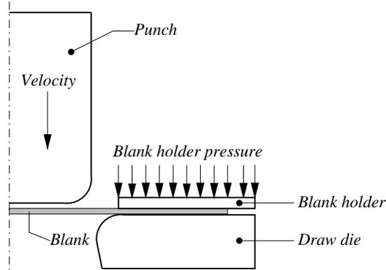
Figure 4. Illustration of the set up of the conventional deep drawing process
