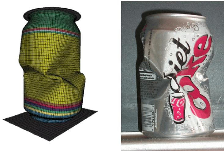
Figure 8. Buckled Deformed Aluminum Can
