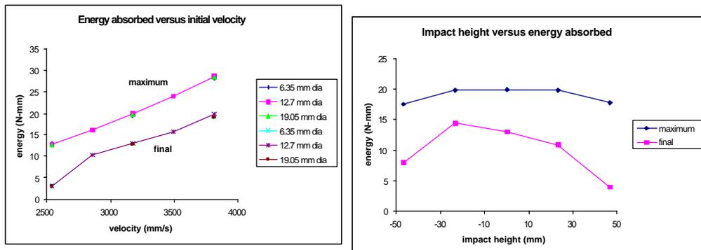
Figure 3. Energy Absorption - Sidewall Indentation
