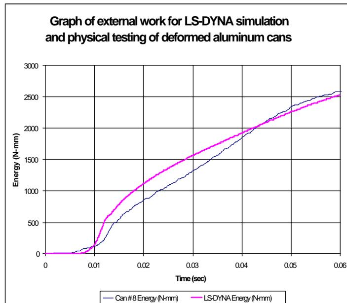
Figure 10. Buckling Energy Curves
