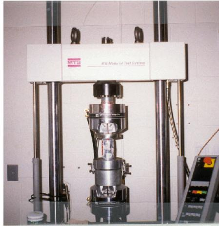
Figure 7. Can Buckling Device
