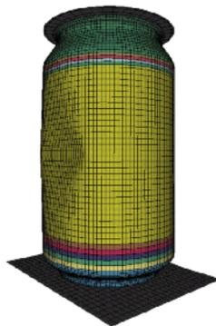
Figure 5. Deformed Can Buckling Model - Initial Condition
