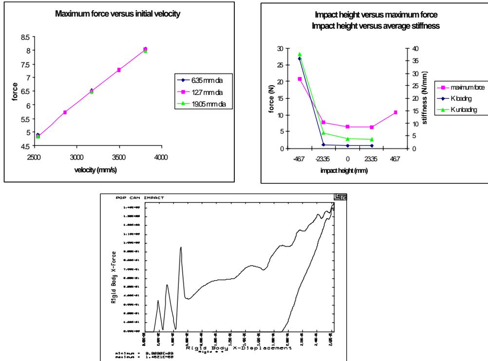
Figure 4. Forces - Sidewall Indentation
