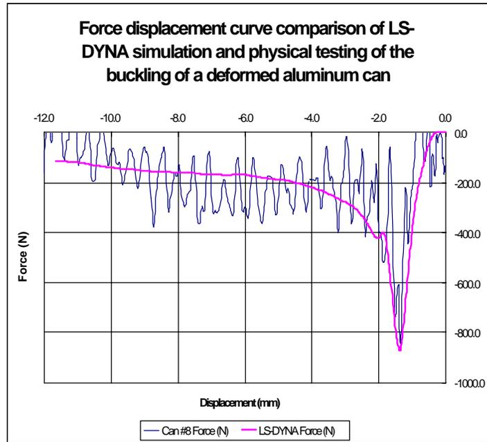
Figure 9. Buckling Force-Displacement
