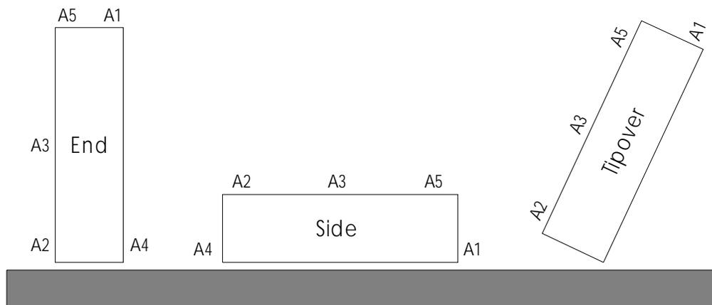
Figure 1. Steel billet test accelerometer locations.
