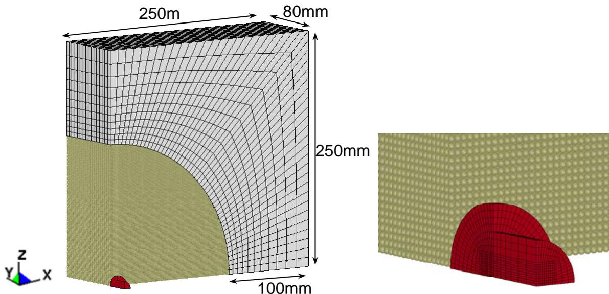
Figure 1: Model Geometry and Close up view of rigid projectile
