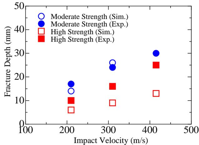
Figure 7: Correlation between fracture depth and impact velocity
