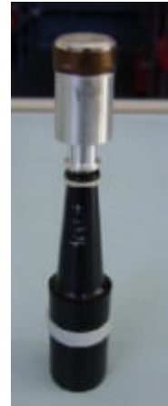
Figure 10: Instrumented ammunition. Strain gauge implemented on the rod (left), complete round with flare (right)
