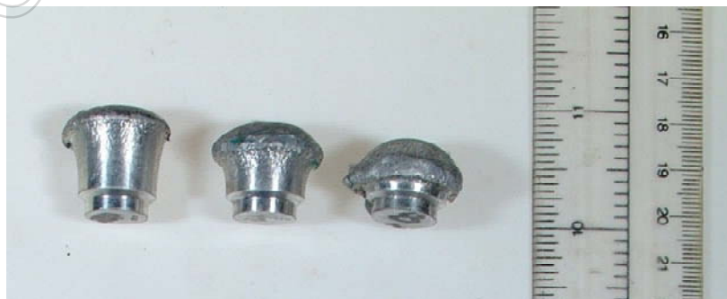
Deformed aluminum projectiles after plate perforation.
