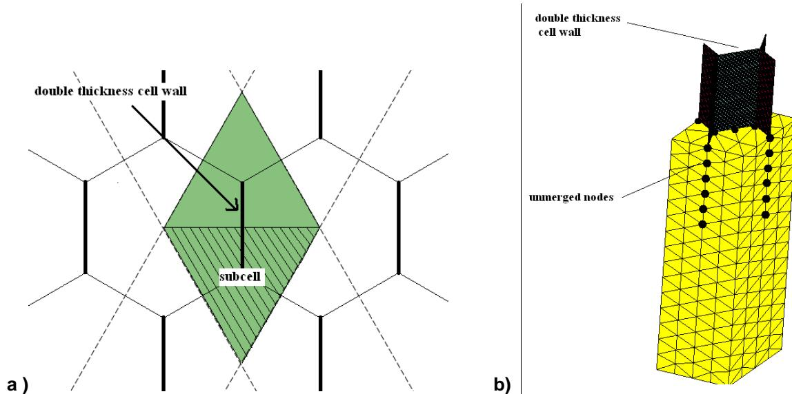
Figure 1 – Hybrid unit cell and subcell models
