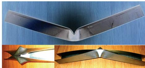
Figure 3: U-section collapse mode for all impact velocities
