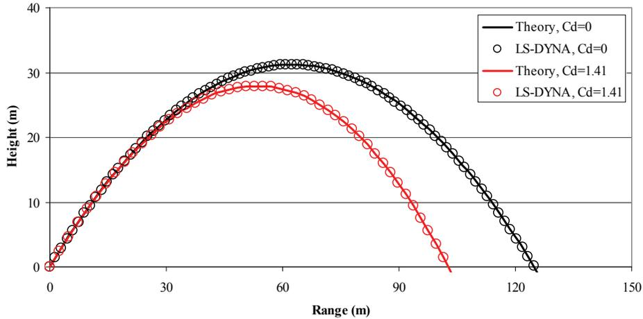
Figure 4: Validation of the air-drag subroutine in LS-DYNA (symbols), result compared to the numerical solution of Eq.2 (solid lines).
