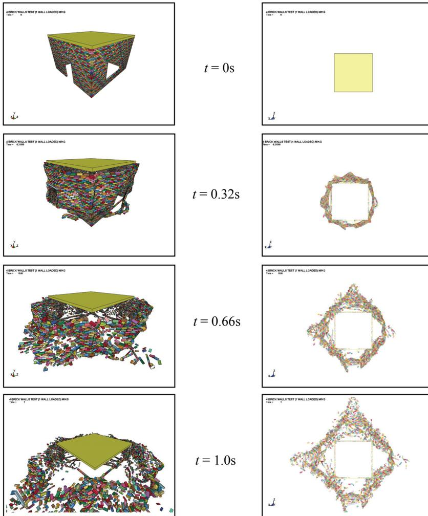
Figure 6 A series of images showing the failure and debris scatter of a building structure
