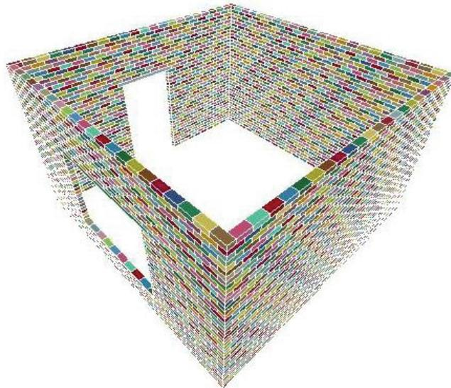
Figure 1: Typical output from FE-WALL software with roof removed for clarity. Model consists of approximately 3000 individual brick parts.
