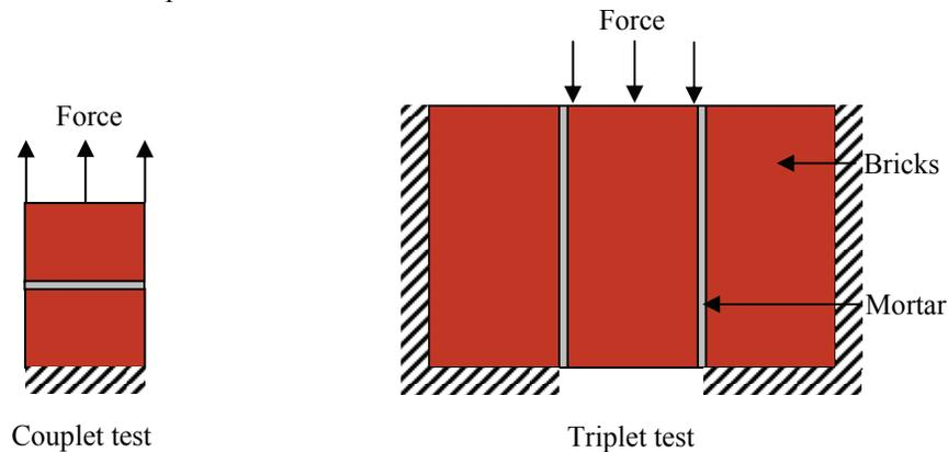
Figure 3: Images showing the setup of the couplet (left) and triplet (right) tests
