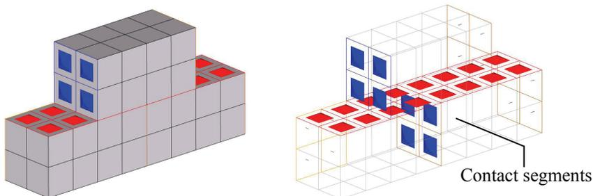
Figure 2: Image showing a subset of bricks with contacts segments (tiebreak) generated automatically with FE-WALL software.
