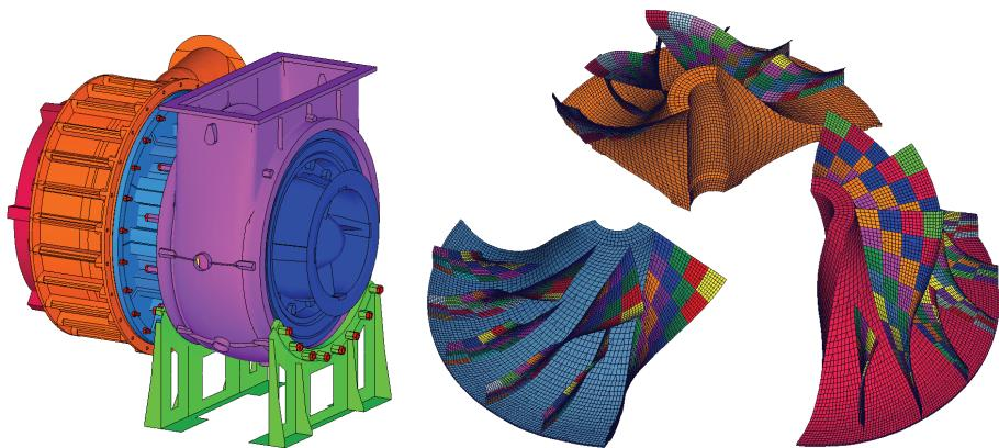
Figure 2: Simulation Model – Entire Turbocharger and Compressor Wheel
