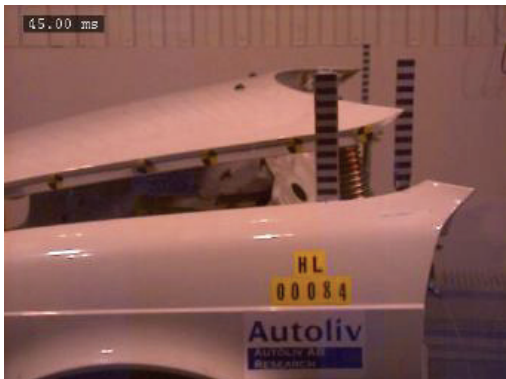
Figure 1 Active hood in activated (lifted) position [3]
