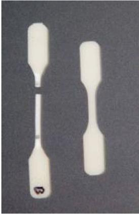
Figure 4: Test specimens showing post-yield necking behavior
