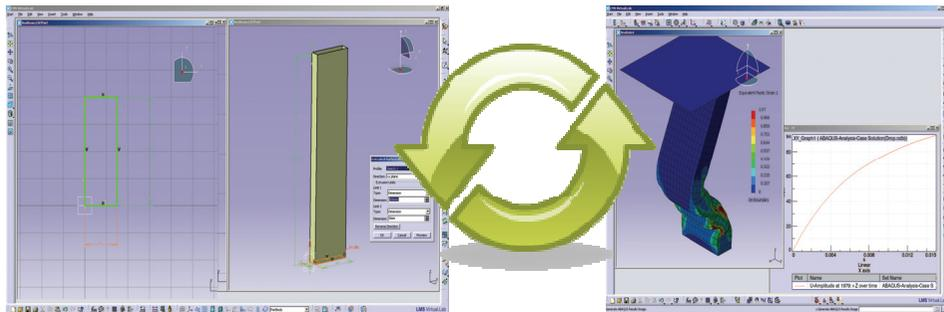
Figure 4: Drop test analysis - Associativity with CAD
