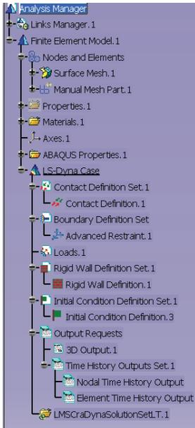
Figure 5: Feature tree of drop test analysis, showing all steps of the process
