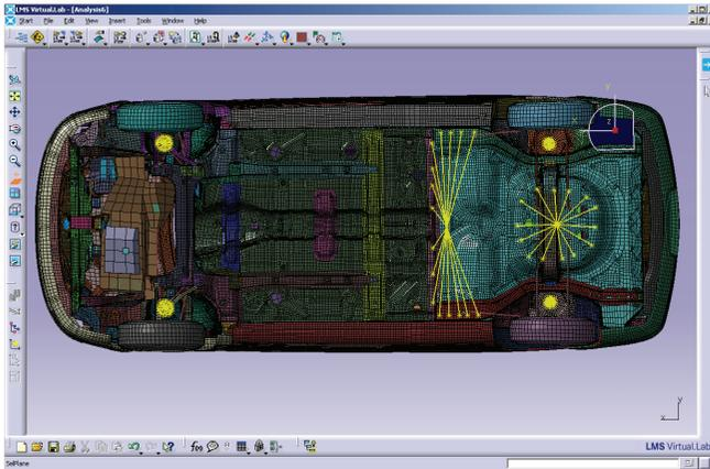
Figure 6: Lumped mass trimming of vehicle.
