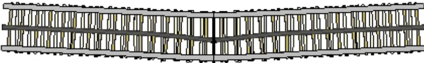
Figure 12: Maximum deformation of reinforcement in Column 2
