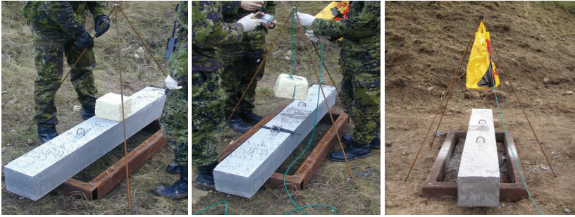
Figure 3: Experimental setup – column, steel frame and high explosive charge
