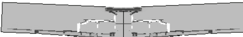
Figure 10: Maximum damage on Column 2 – aramid lacing for every 100mm
