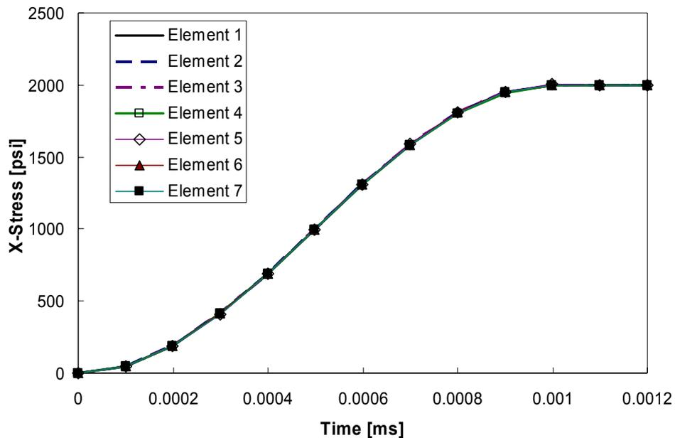
Figure 3 Demonstration of analytical solution obtained for x-stress component using fully integrated S/R (ELFORM=2) 8-node hexahedral solid element.
