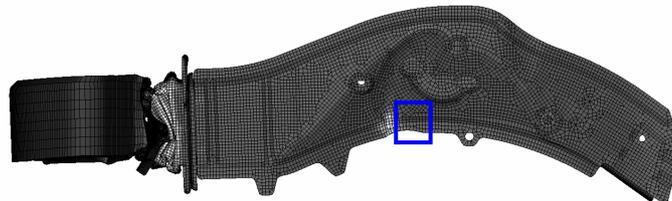
Figure 8 Fringe plot of the plastic strain. The maximum value in the crash beam is used as a response. The maximum value is found inside the box in the picture
