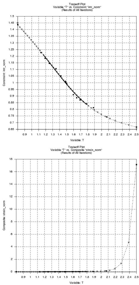
**Figure 4 Trade-off curve when varying the sheet thickness, the intrusion to the left and the plastic strain to the right. The square markers are all simulated values.**
