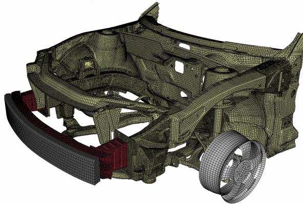
**Figure 6 The vehicle model**
