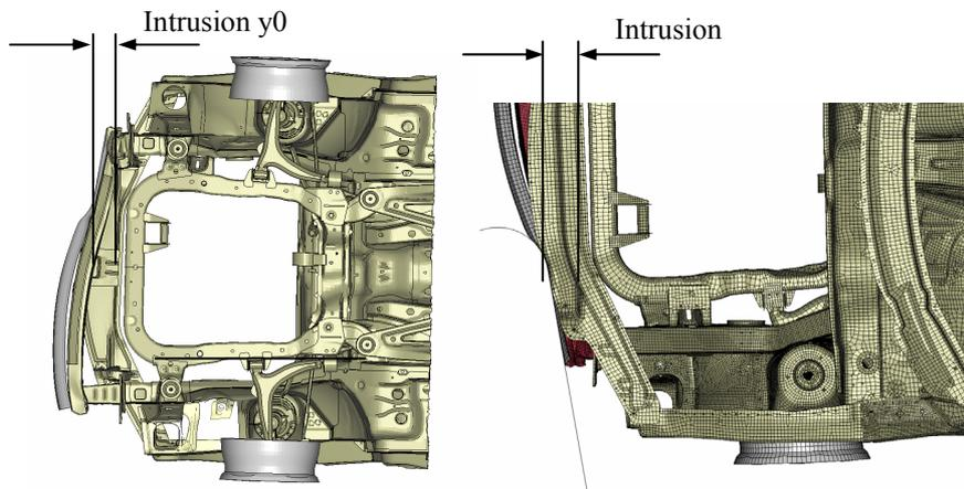
Figure 7 Bottom and top views of the maximum deformation
