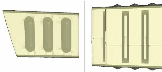
**Figure 17 The geometry of the crash-box in the optimal design point.
