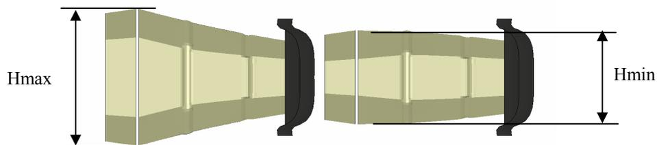
**Figure 3 The change in height of the small FE model**
