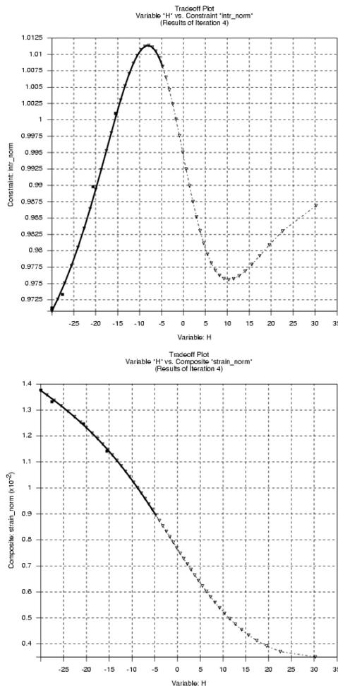
**Figure 5 Trade-off curve when varying the height of the box, the intrusion to the left and the plastic strain to the right. The square markers are all simulated values.**
