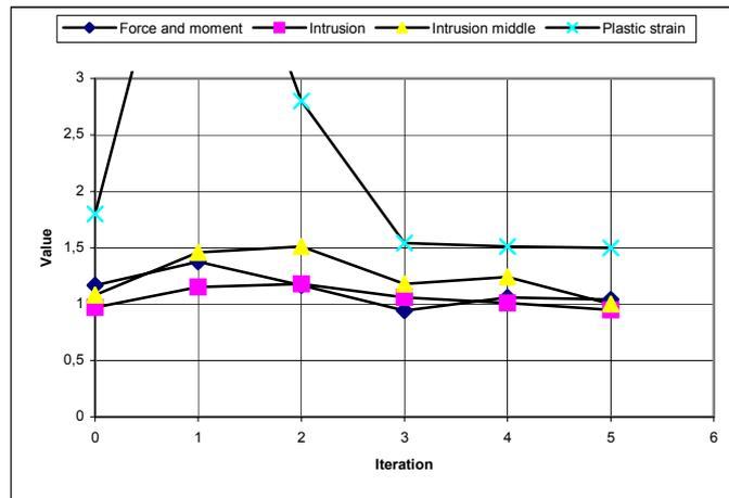
Figure 15 Optimization of all constraints. The upper limit is equal to one for all constraints
