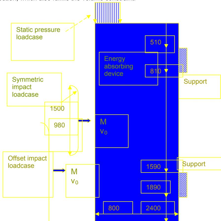
Fig.1. Ground structure of the energy absorbing device. Length unit mm.
