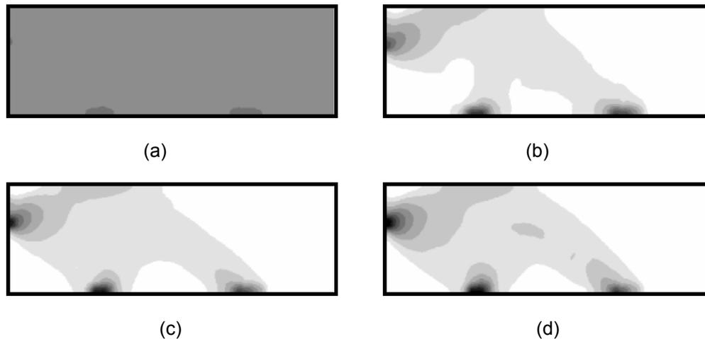
Fig.3. Pressure loading case. Thickness distribution after 2 (a), 10 (b), 18 (c), and 26 (d) iterations
