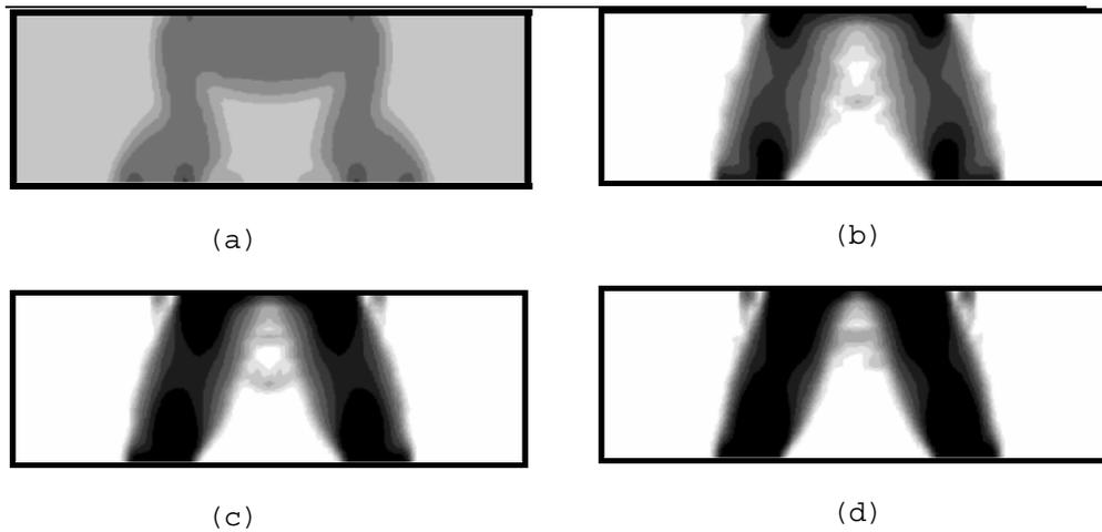
Fig.2. Symmetric impact case. Thickness distribution after 2 (a), 8 (b), 16 (c), and 26 (d) iterations
