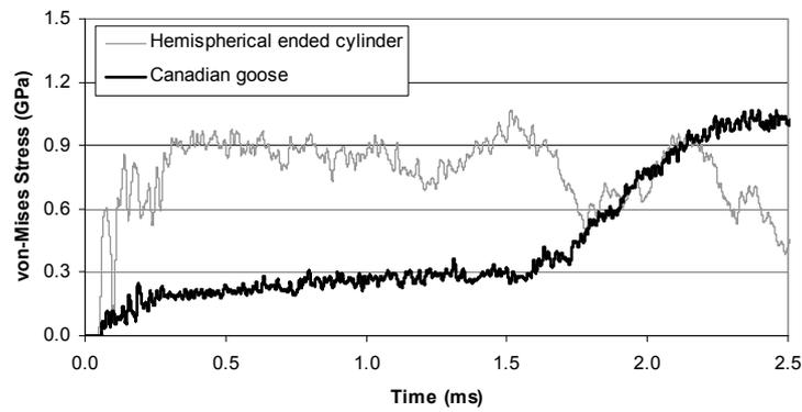
Figure 8 von-Mises stress (centre of panel target) predicted for the impact of a multi-material model, compared to the hemi-spherical ended cylinder.
