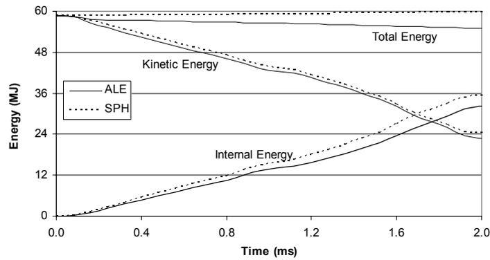
Figure 2 Variation in global energy resulting from the impact of a hemi-spherical ended cylinder into a square flat panel.
