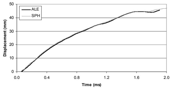
Figure 5 Resultant displacement (centre of target) predicted for the impact of a hemi-spherical ended cylinder into a square flat panel.
