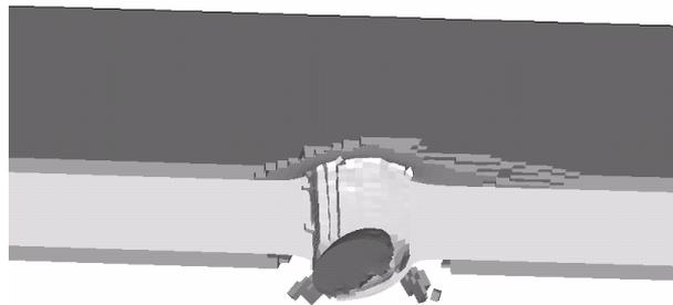
Figure 5 – Orbital debris impact against a CRFP/aramidic-fibres/CRFP panel
