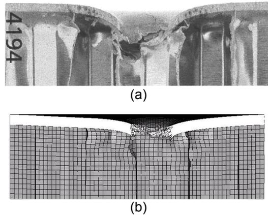
Figure 1 – Low velocity impact test: qualitative comparison between (a) experimental data and (b) numerical results
