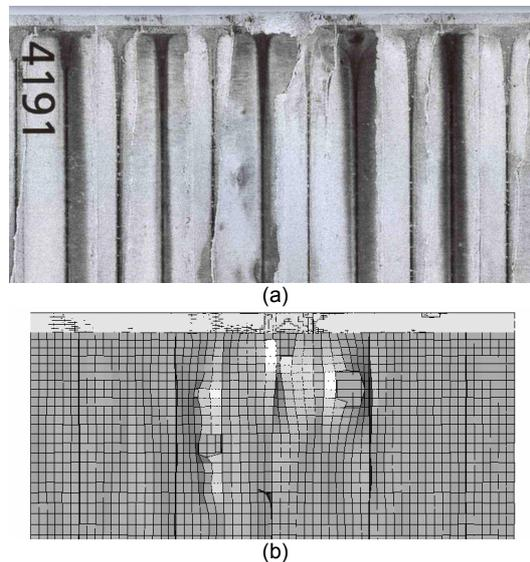
Figure 2 – High velocity impact test: qualitative comparison between (a) experimental data and (b) numerical results
