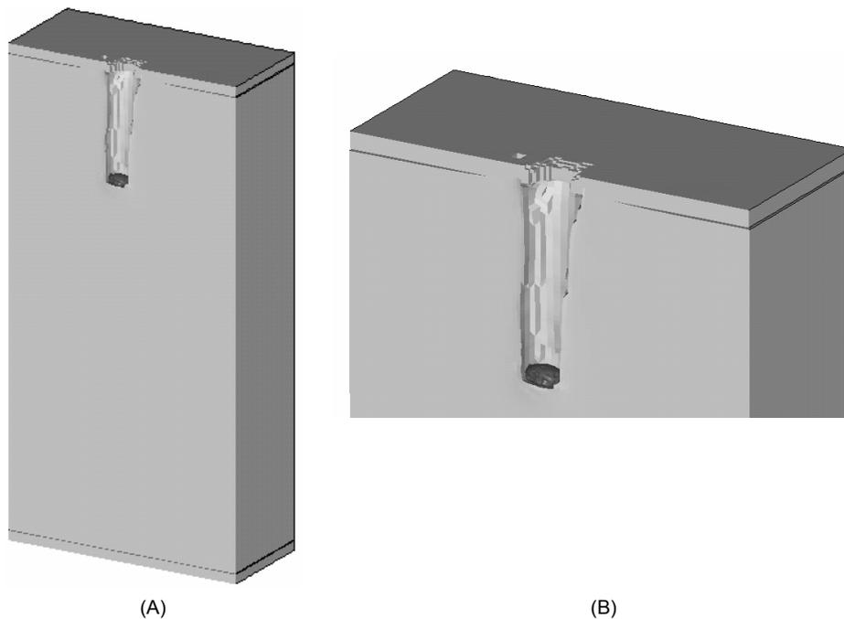
Figure 3 –Orbital debris impact against a sandwich panel with polymeric foam core.
