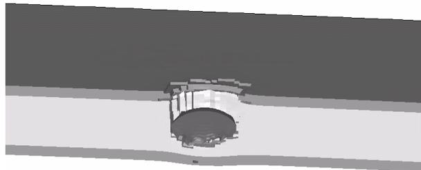
Figure 4 – Orbital debris impact against an Aluminium/aramidic-fibres/Aluminium panel
