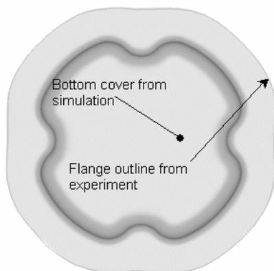
Figure 2: A comparison of the simulation results with measurements for the pump component. The line L along which some of the measurements are done is shown in Figure 1.
