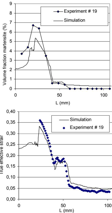
Figure 3: A comparison of the simulation results with measurements for the pump component. The line L along which some of the measurements are done is shown in Figure 1.
