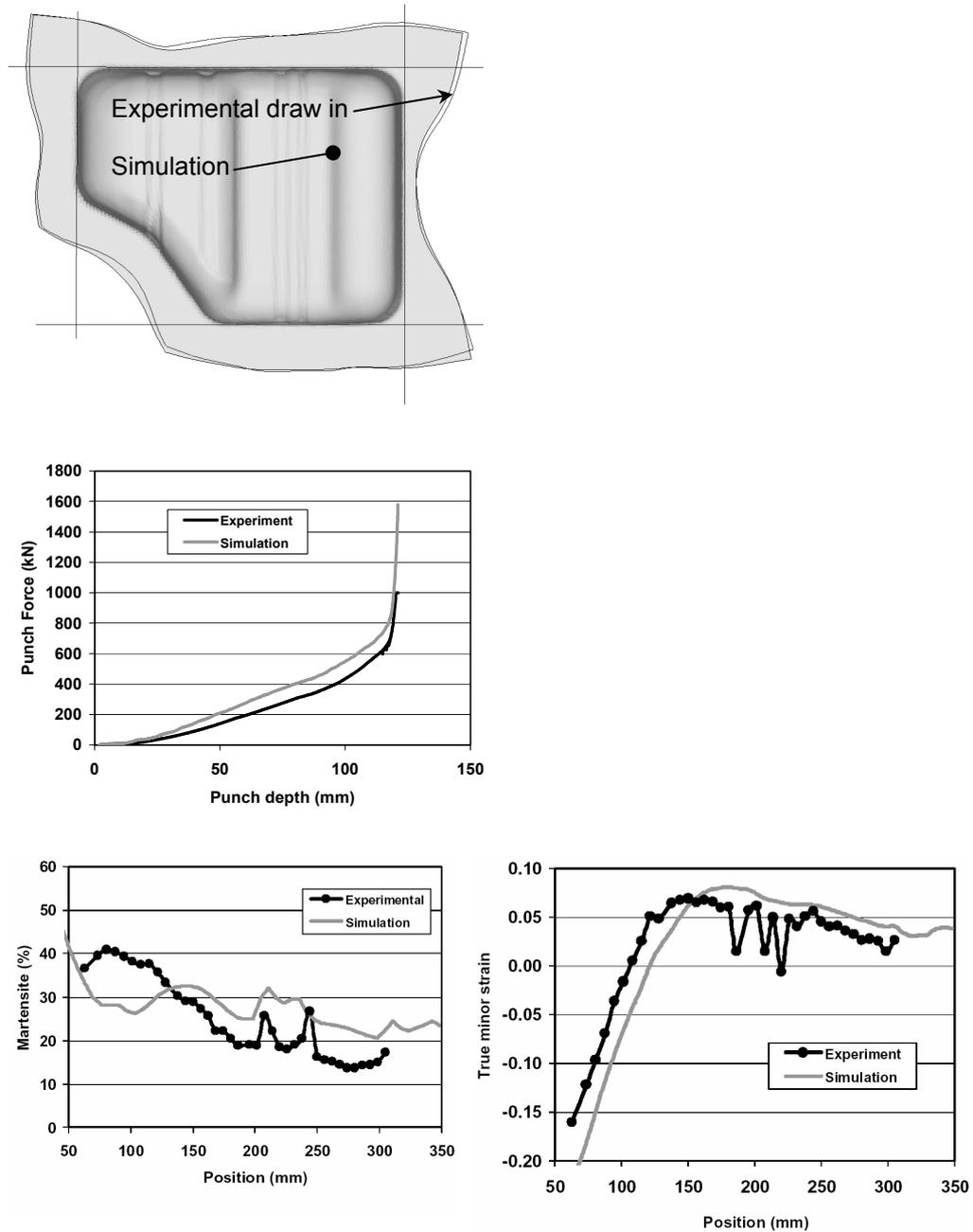
Figure 5: A comparison of the simulation results with measurements for the muffler component. The line A along which some of the measurements are done is shown in Figure 4.
