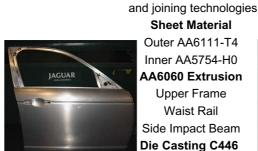
**Sheet Material** Outer AA6111-T4 Inner AA5754-H0 AA6060 Extrusion Upper Frame Waist Rail Side Impact Beam **Die Casting C446** Hinge Reinf. Panel
