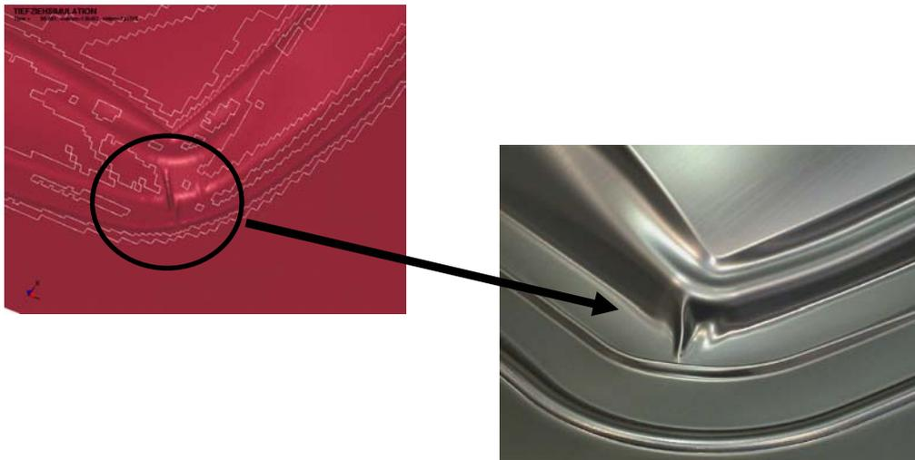
**Figure 1:** Wrinkles in the simulation (left) and on the real part (right)
