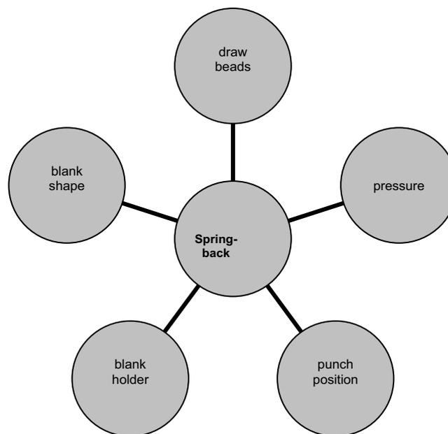
**Figure 3:** Parameters which influence the spring-back behaviour
