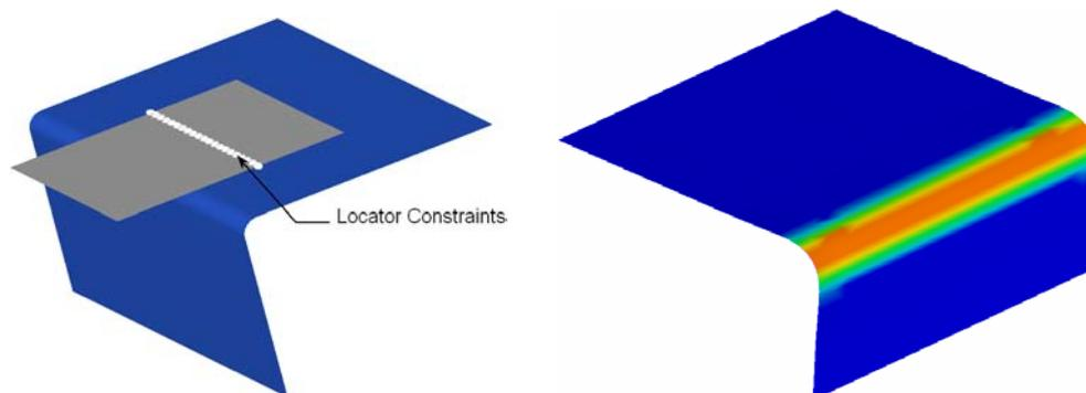
**Figure 4(a)** Simulation Setup - In plane motion of the blank was constrained to simulate the effect of locator pins
