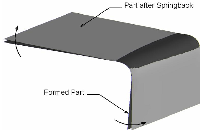
**Figure 5** Overlay of Formed Part and Part after Springback
