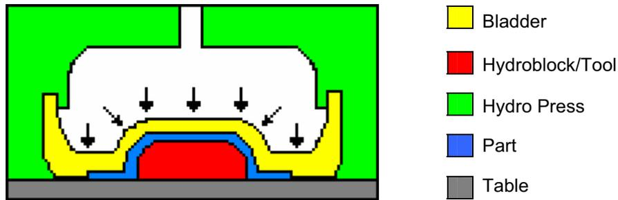
**Figure 1** Schematic Transverse Section of the ASEA Bladder Hydro Press
