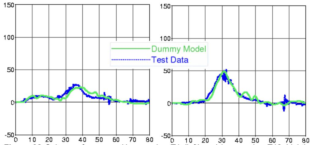
**Figure 32** Spine performance: Upper spine T1 (left) and lower spine T12 (right); graphs show acceleration [g] vs. time [ms]
