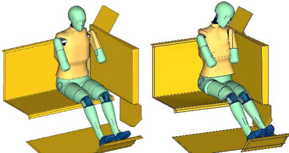
**Figure 10** Dummy model before (right) and during impact (left)
