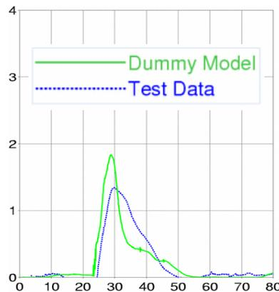
**Figure 29** Abdominal resultant force; graph shows force [kN] vs. time [ms]
