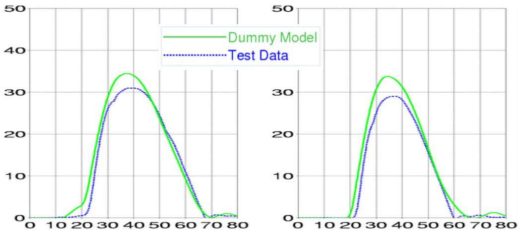
**Figure 26** Rib performance: Middle rib (left) and lower rib (right); graphs show deflection [mm] vs. time [ms]
