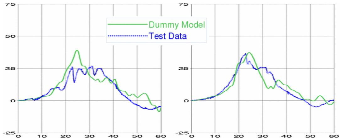
**Figure 38** Spine performance: Upper spine (left) and lower spine (right); graphs show acceleration [g] vs. time [ms]
