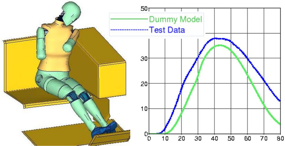
**Figure 30** Dummy model during impact (left) and performance of upper rib (right); graph shows intrusion [mm] vs. time [ms]
