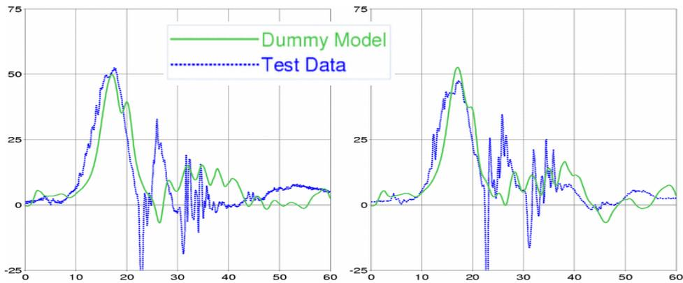
**Figure 37** Rib performance: Upper rib (left) and lower rib (right); graphs show acceleration [g] vs. time [ms]
