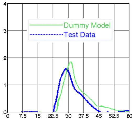
**Figure 23** Abdominal resultant force; graph shows force [kN] vs. time [ms]
