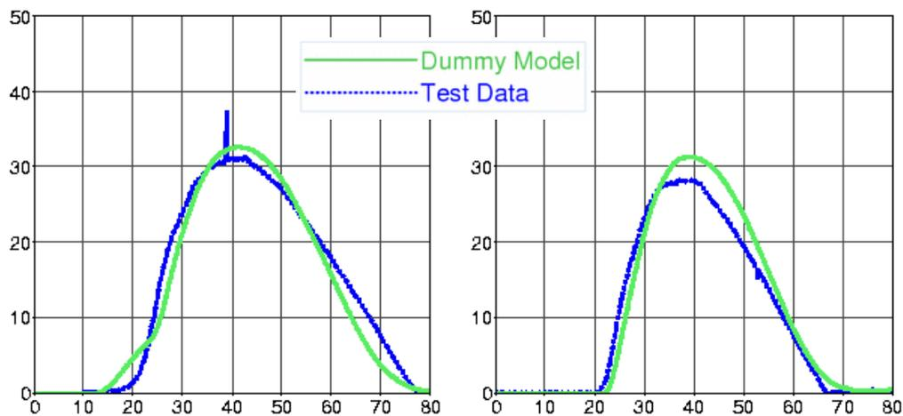
**Figure 31** Rib performance: Middle rib (left) and lower rib (right); graphs show deflection [mm] vs. time [ms]
