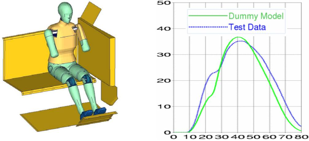
**Figure 25** Dummy model before impact (left) and performance of upper rib (right); graph shows intrusion [mm] vs. time [ms]
