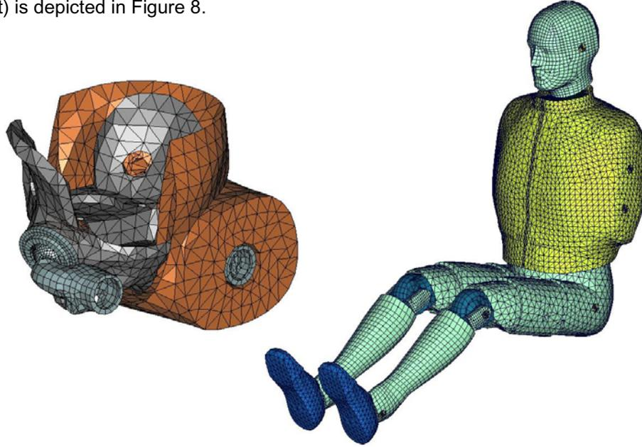
**Figure 8** FAT USSID model; cut of pelvis model (left), complete model (right)
