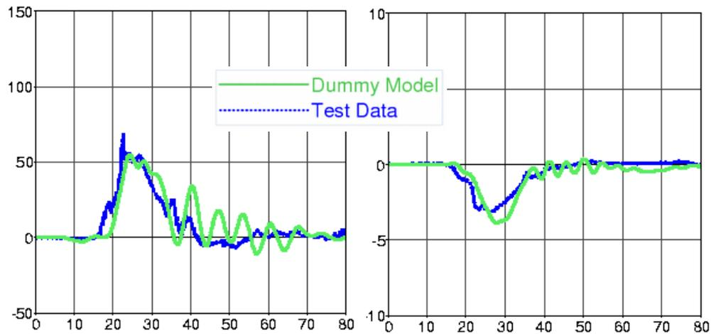
**Figure 33** Pelvis performance: Pelvis accelerations (left) and pubic symphysis force (right); graphs show acceleration [g] vs. time [ms] and force [kN] vs. time [ms], respectively
