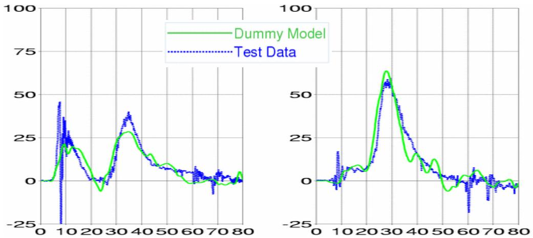
**Figure 27** Spine performance: Upper spine T1 (left) and lower spine T12 (right); graphs show acceleration [g] vs. time [ms]
