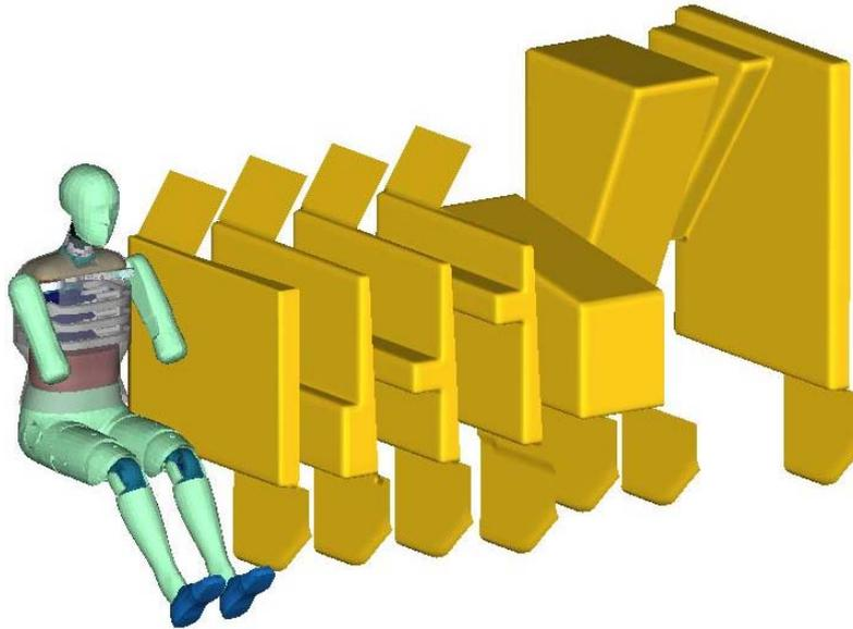
**Figure 2** Barrier shapes used to validate FAT EUROSID-1 and USSID model
