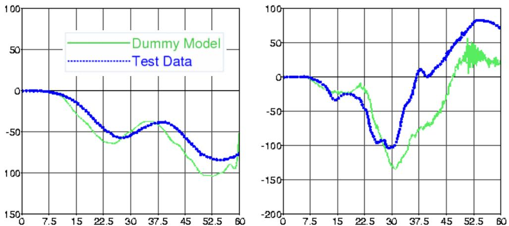
**Figure 25** X-Moment of Force transducer T1 (left) and T12 (right); graphs show moment [Nm] vs. time [ms]
