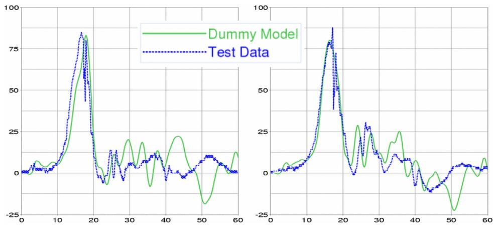
**Figure 40** Rib performance: Upper rib (left) and lower rib (right); graphs show acceleration [g] vs. time [ms]
