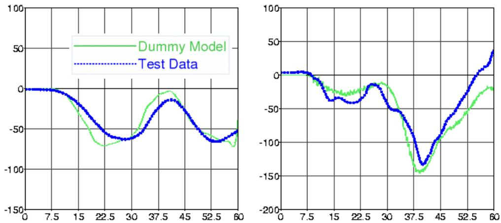
**Figure 18** X-Moment of Force transducer T1 (left) and T12 (right); graphs show moment [Nm] vs. time [ms]
