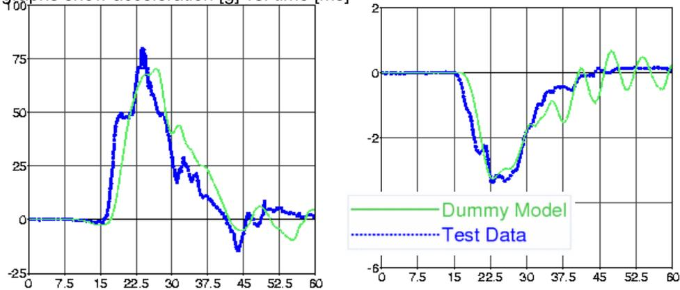
**Figure 22** Pelvis performance: Pelvis accelerations (left) and pubic symphysis force (right); graphs show acceleration [g] vs. time [ms] and force [kN] vs. time [ms], respectively
