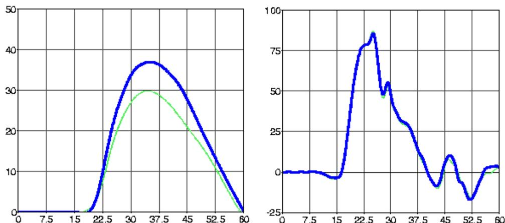
**Figure 6** Rib intrusion of middle rib (left) and pelvis acceleration (right) of ES-2 in a sled test with different frictional parameters for the dummy to dummy contact; the graphs show [mm] and [g] vs. time [ms], respectively
