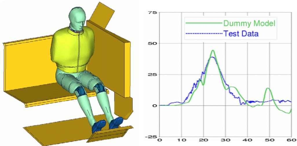
**Figure 36** Dummy model before impact of plane barrier (left) and performance of pelvis (right); graph shows acceleration [g] vs. time [ms]
