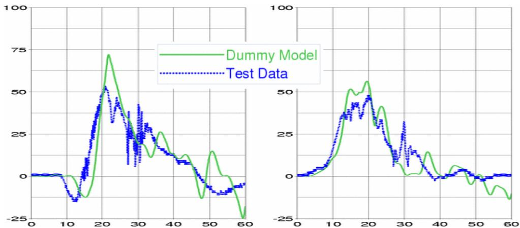
**Figure 41** Spine performance: Upper spine (left) and lower spine (right); graphs show acceleration [g] vs. time [ms]
