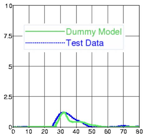
**Figure 34** Abdominal resultant force; graph shows force [kN] vs. time [ms]
