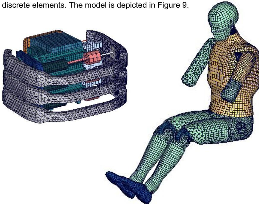
**Figure 9** FAT ES-2 model; rib assembly (left), assembled model (right)
