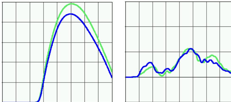
**Figure 5** Rib intrusion and upper spine acceleration of ES-2 dummy barrier height of barrier depicted in Figure 19; barrier height for green curve 20 mm higher
