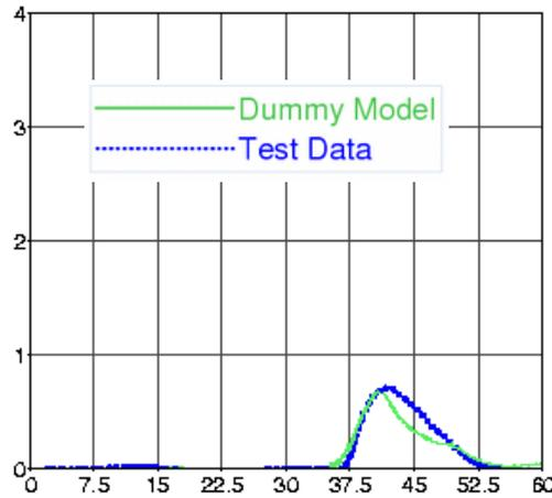
**Figure 16** Abdominal resultant force; graph shows force [kN] vs. time [ms]
