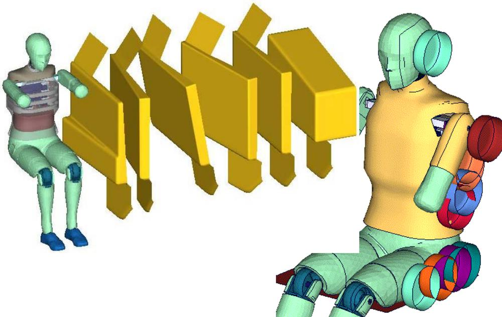
**Figure 3** Barrier shapes (left) and pendulum impact locations (right) used to validate the FAT ES-2 model
