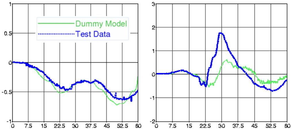
**Figure 24** Y-Force of force transducer T1 (left) and T12 (right); graphs show force [kN] vs. time [ms]
