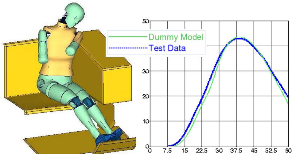
**Figure 19** Dummy model during impact (left) and performance of upper rib (right); graph shows intrusion [mm] vs. time [ms]
