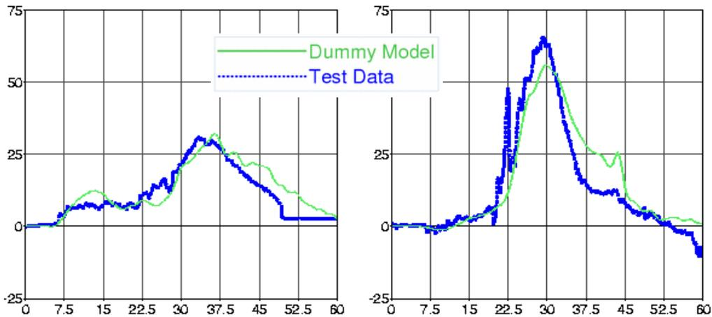
**Figure 21** Spine performance: Upper spine T1 (left) and lower spine T12 (right); graphs show acceleration [g] vs. time [ms]
