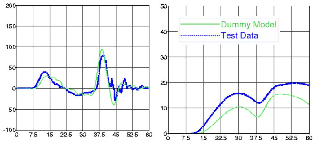
**Figure 11** Upper rib acceleration and intrusion. Graphs show acceleration [g] and deflection [mm] vs. time [ms], respectively
