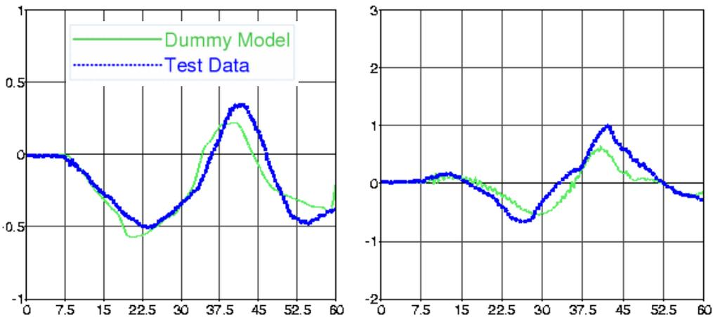
**Figure 17** Y-Force of force transducer T1 (left) and T12 (right); graphs show force [kN] vs. time [ms]
