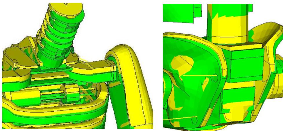
**Figure 4** ES-2 dummy parts as obtained by meshing CAD data in yellow and model under gravity load in green; Upper thorax (left), sacrum block (right)
