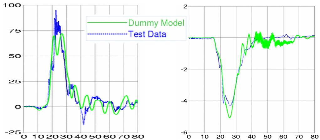
**Figure 28** Pelvis performance: Pelvis accelerations (left) and pubic symphysis force (right); graphs show acceleration [g] vs. time [ms] and force [kN] vs. time [ms], respectively
