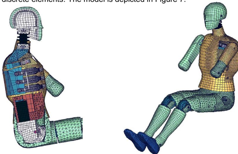
**Figure 7** FAT Eurosid-1 model; cut (left), complete model (right)
