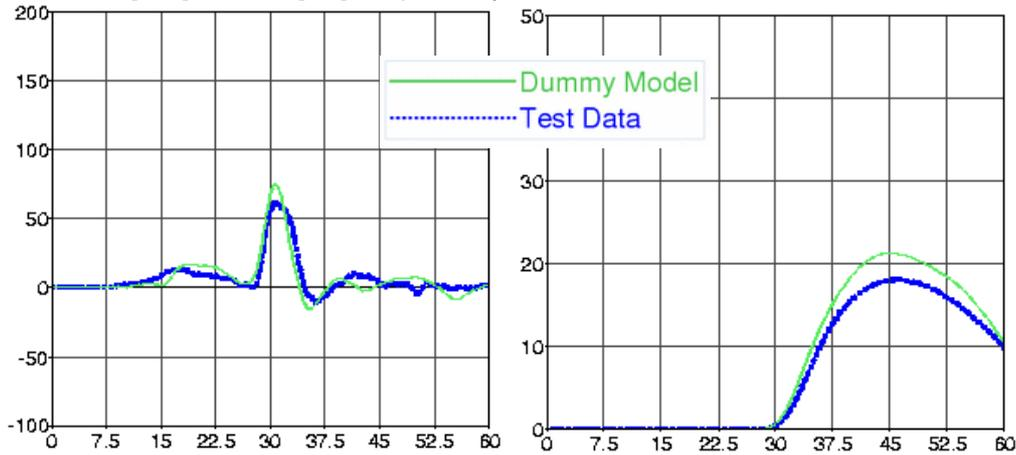
**Figure 13** Upper rib acceleration and intrusion; graphs show acceleration [g] and deflection [mm] vs. time [ms], respectively
