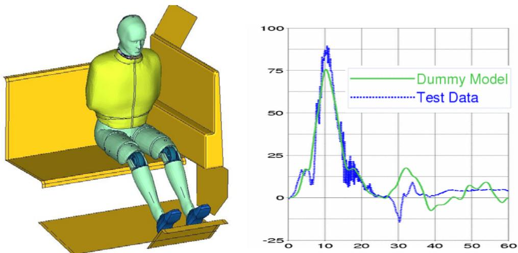
**Figure 39** Dummy model before impact with barrier with pelvis impactor (left) and performance of pelvis (right); graph shows acceleration [g] vs. time [ms]
