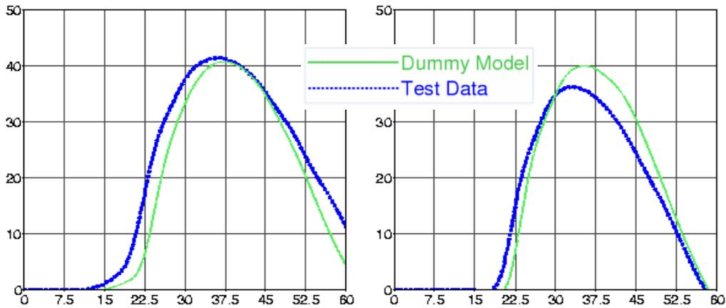
**Figure 20** Rib performance: Middle rib (left) and lower rib (right); graphs show deflection [mm] vs. time [ms]
