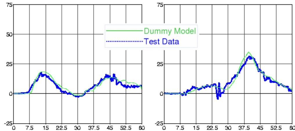
**Figure 14** Spine performance: Upper spine T1 (left) and lower spine T12 (right); graphs show acceleration [g] vs. time [ms]
