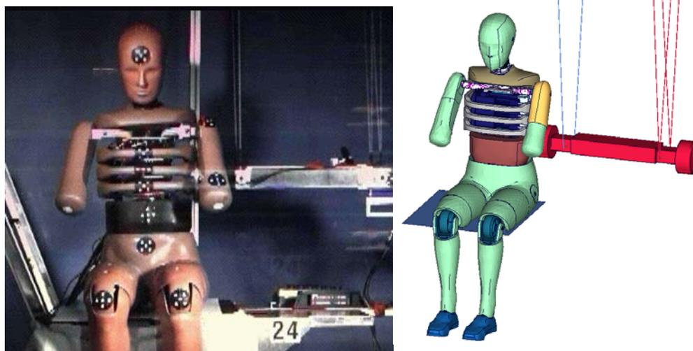
**Figure 1** Dummy (left) and model (right) in pendulum test
