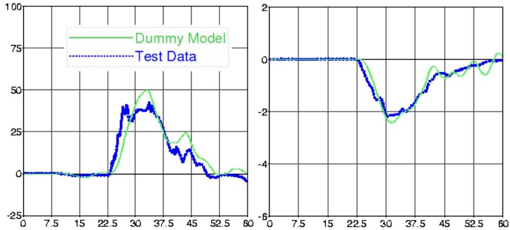
**Figure 15** Pelvis performance: Pelvis accelerations (left) and pubic symphysis force (right); graphs show acceleration [g] vs. time [ms] and force [kN] vs. time [ms], respectively
