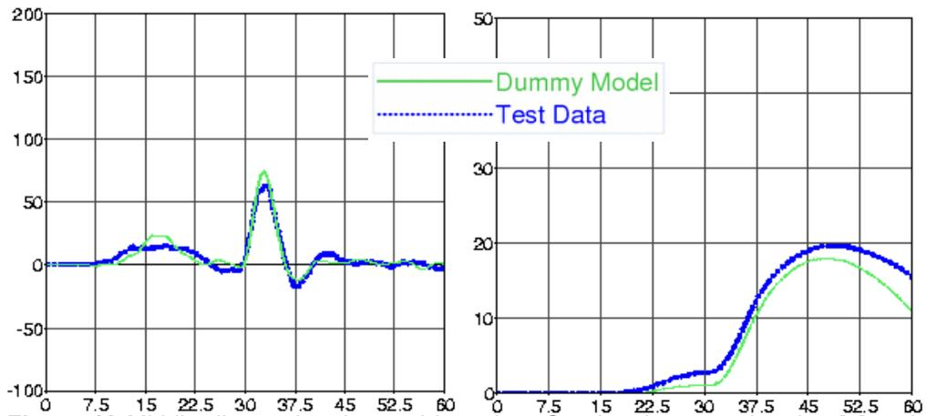
**Figure 12** Middle rib acceleration and intrusion. Graphs show acceleration [g] and deflection [mm] vs. time [ms], respectively
