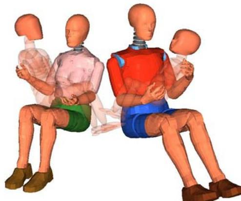
Development programs have been performed in co-operation with several industrial partners. Based on actual OOP applications, component and full dummy validation sets with representative loading severity and loading rate have been gathered. The thorax and the neck are the most critical components for OOP simulation. This justified the introduction of full FE models of the dummy thorax. For the neck a detailed multibody approach was found to be most robust and accurate.
