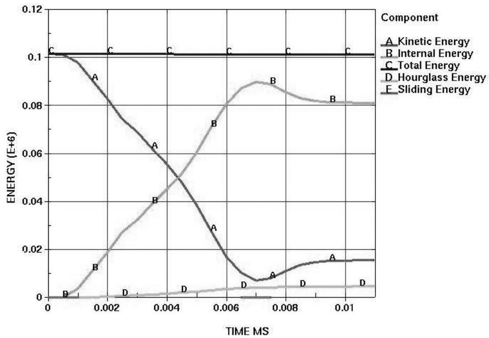
Figure 7: Energy balance for the 20 mm cone height simulation.
