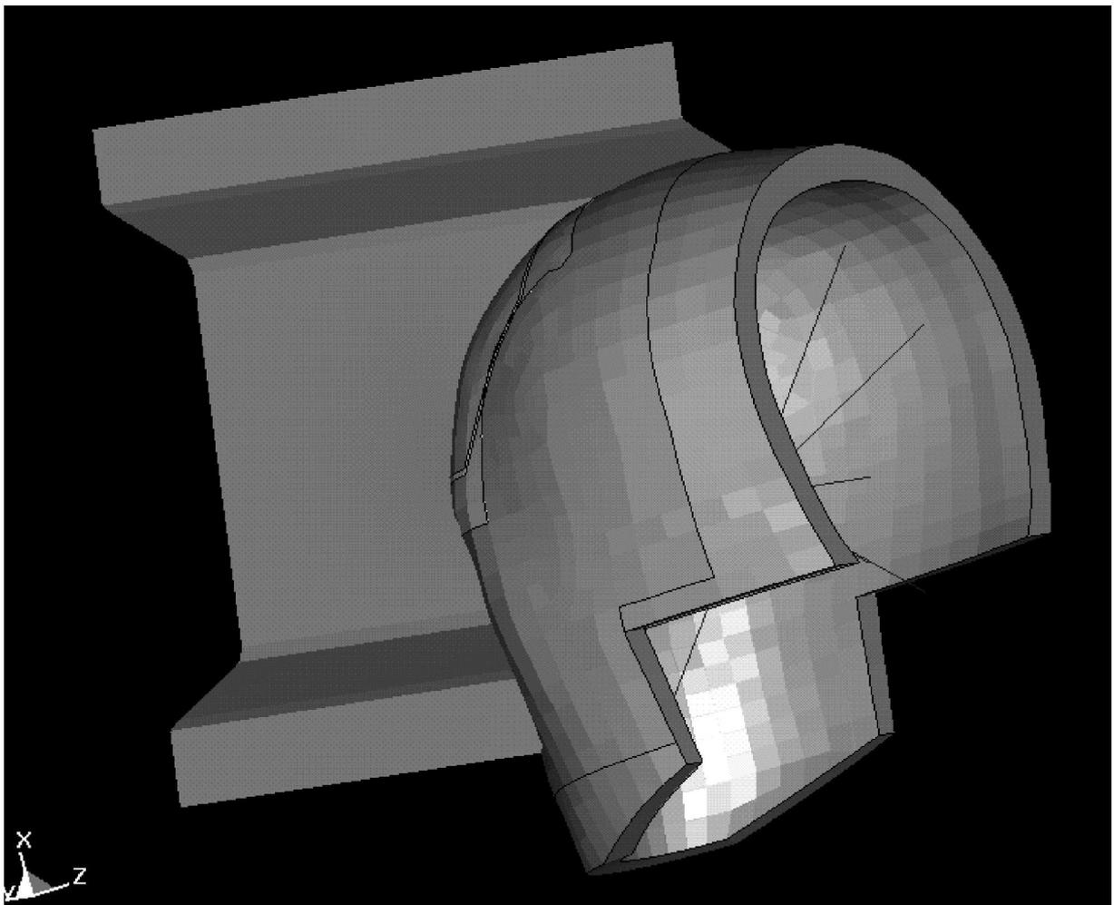
**Figure 1: Baseline model with the Free Motion Headform impacting the hat sectioned sheet metal**
