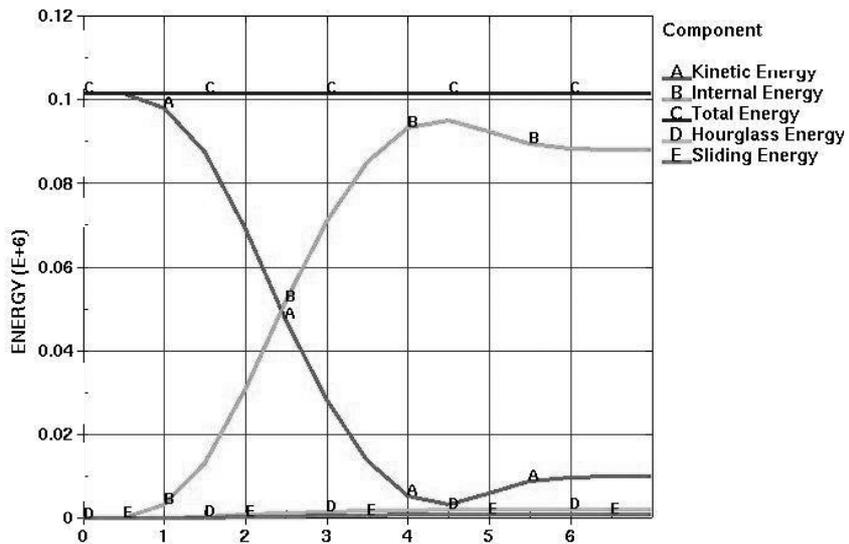
**Figure 3: Energy balance plot for the baseline model.**
