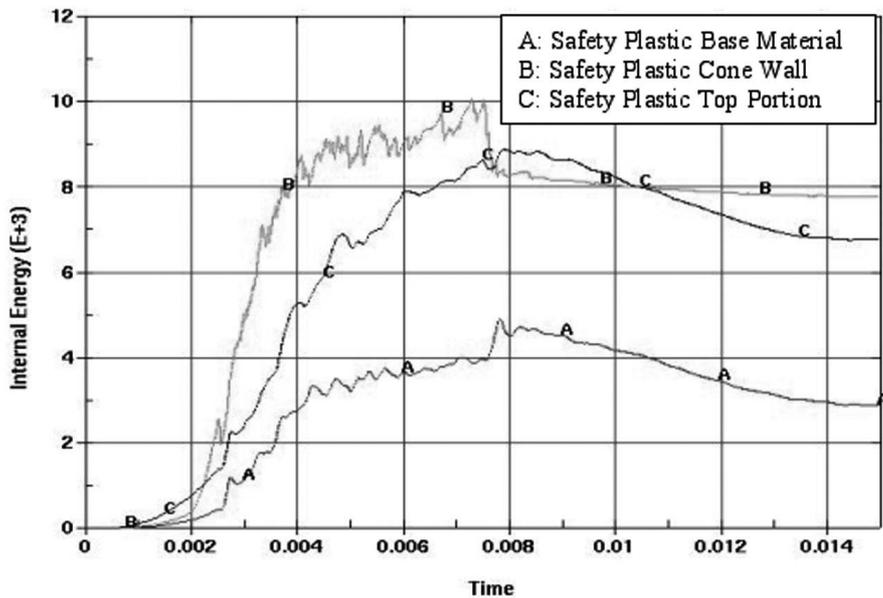
**Figure 10: Internal Energy plot for 20mm cone height with 0.04 inch initial thickness.**
