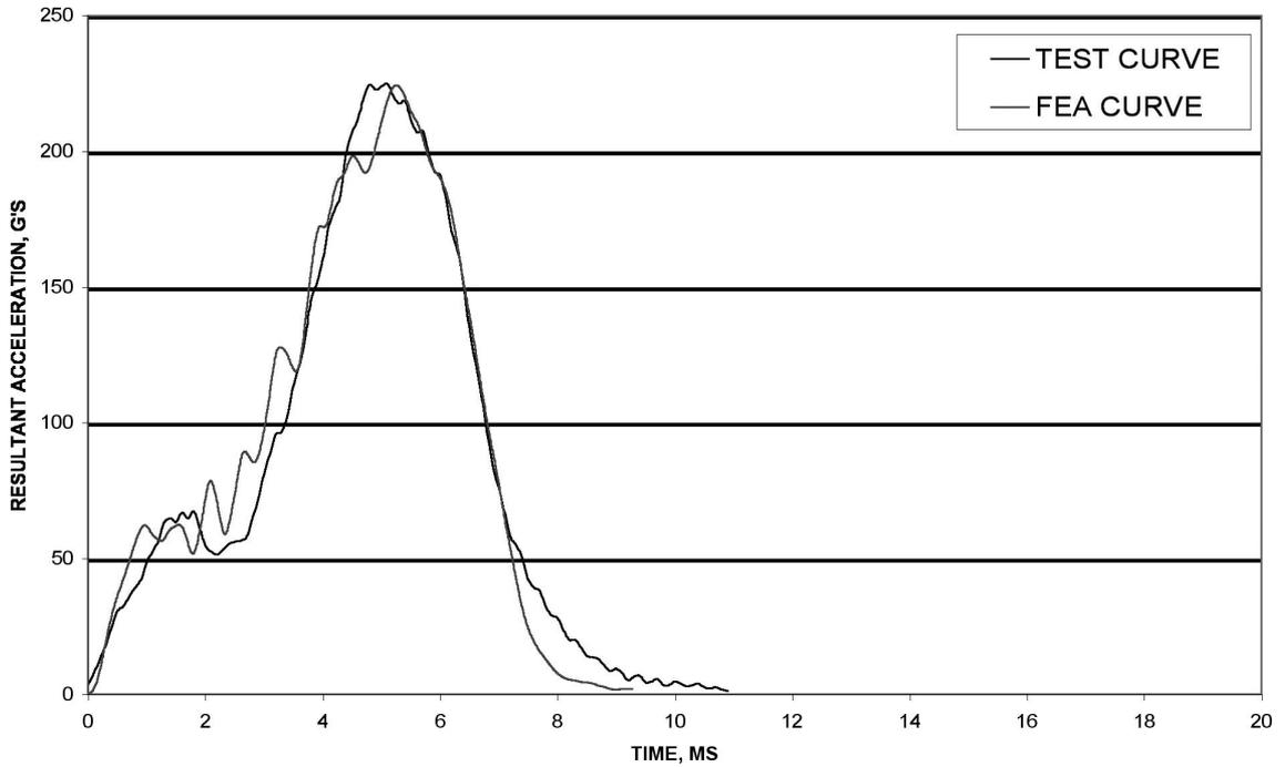
Figure 8: Comparison of acceleration Vs time curves for 14.5 mm cone height with 0.04 inch initial thickness of the safety plastic.
