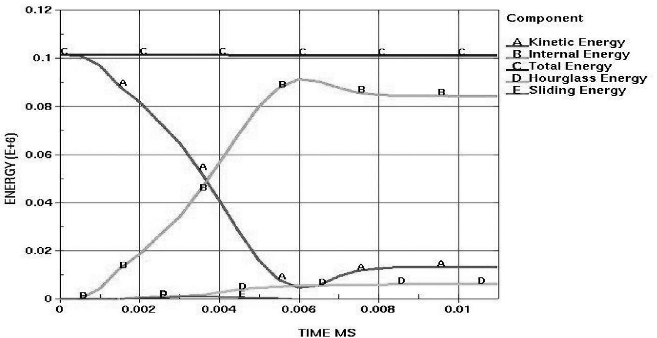
Figure 9: Energy balance plot for 14.5mm cone height
