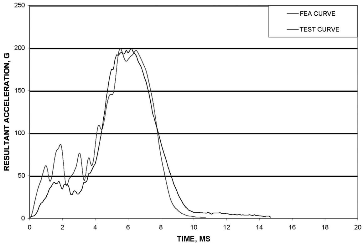
Figure 6: Comparison of acceleration Vs time curves for 20 mm cone height and 0.04 inch initial thickness of the safety plastic.
