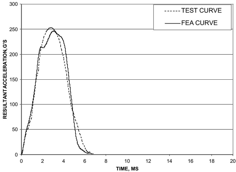
**Figure 2. Comparison of acceleration Vs time curves for the baseline model.**
