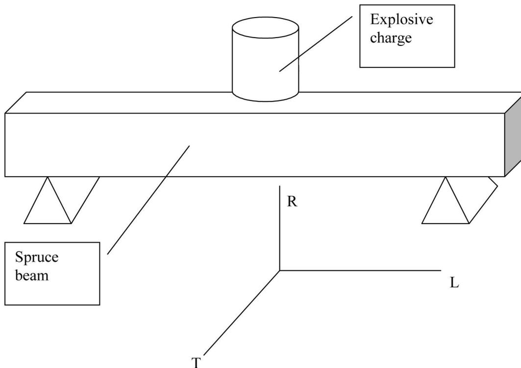
**Fig.1. Schematic of the Spruce beam loading.**
