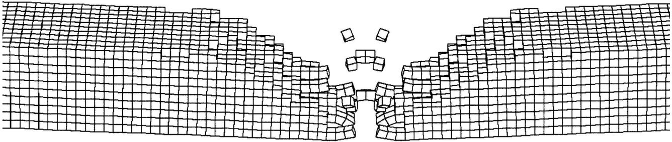
**Fig. 5: Damage of the Spruce beam at the time 1 ms.**
