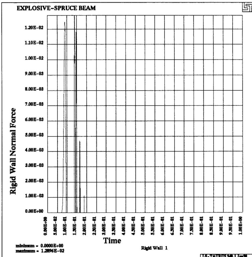
Fig.10. Dependence of the force ( in kN) acting on the beam support on the time ( in ms).
