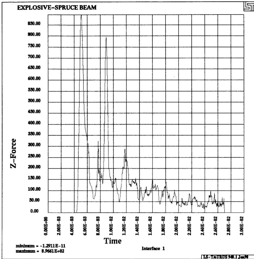
Fig.9. The dependence of the resulting force(in kN) in the contact area on the time (in ms).
