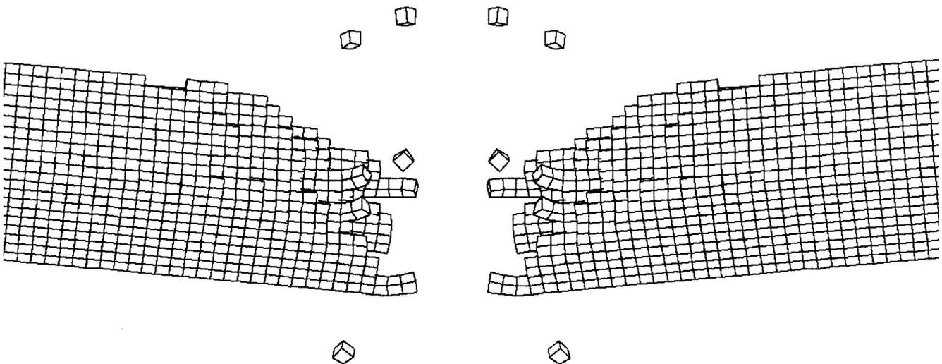
**Fig.7. Damage of the Spruce beam at the time 3 ms.**
