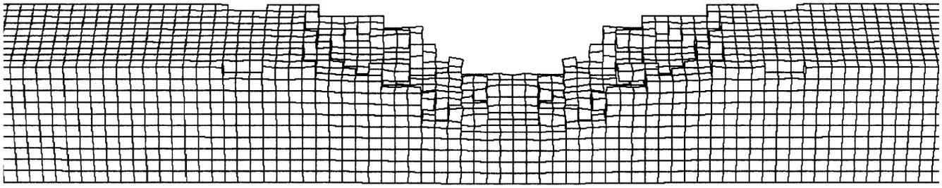
**Fig.4. Damage of the spruce beam at the time 50 ms.**
