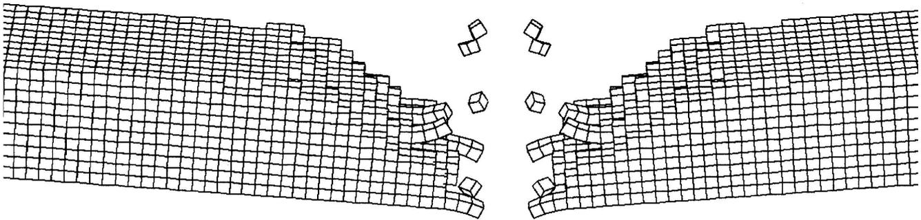
**Fig.6. Damage of the Spruce beam at the time 2 ms.**
