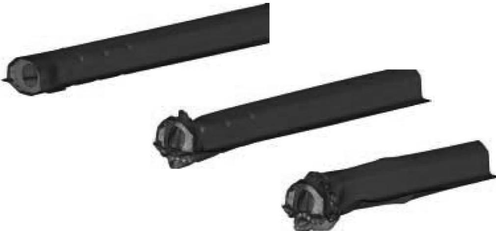
**Figure 16** Longitudinal girder model under crash loading; deformation states; continuum spotweld model
