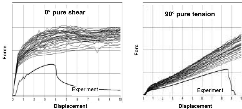
**Figure 9 Measured spotweld forces vs. displacement varying the relative location of the continuum spotwelds; 0° (left, pure shear) and 90° (right, pure tension) loading**
