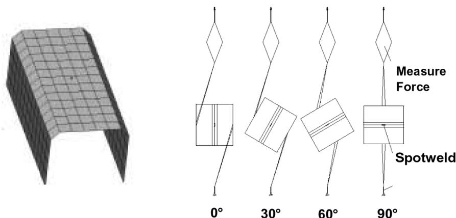
Figure 4 Numerical model for single spotweld connection; FE mesh (left) and general loading model (right) with variation of loading angle
