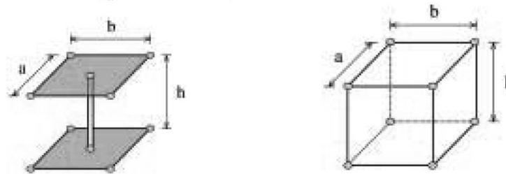
Figure 3 Contact shell set for spotweld modeling (left), Continuum element as spot-weld (right)
