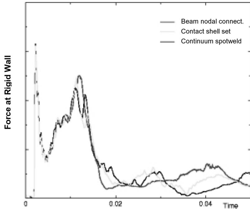
**Figure 17 Longitudinal girder model under crash loading; comparison of time history for longitudinal force of three spotweld models**
