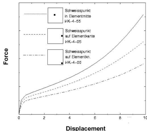
Figure 11 Multiple spotweld example; deformation pattern (left); measured spotweld forces vs. deformation for varied location of the spotweld nodes for nodal connections (right); 0° (pure shear) loading
