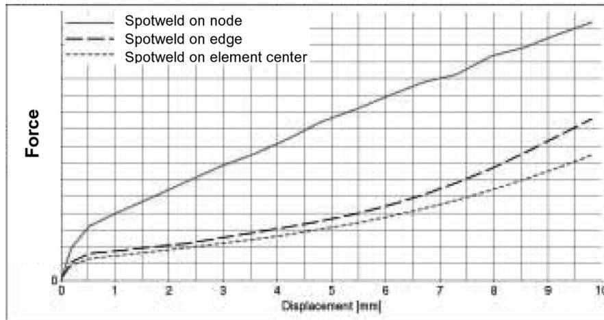
**Figure 12 Measured spotweld forces vs. displacement for varied location of the spot-weld nodes for continuum spotwelds; 0° (pure shear) loading**
