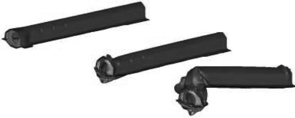
**Figure 14** Longitudinal girder model under crash loading; deformation states; nodal spotweld model
