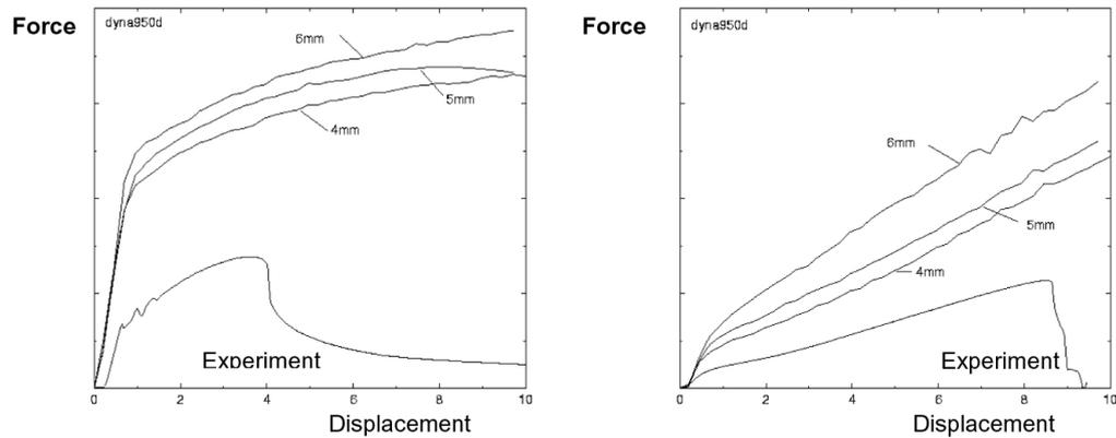
**Figure 8 Measured spotweld forces for varied mesh density (element size 4/5/6 mm) of the spotweld nodes for contact shell sets; 0° (left, pure shear) and 90° (right, pure tension) loading**
