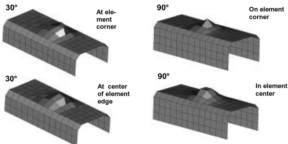
Figure 7 Deformation of single spotweld connection for nodal spotweld model; variation of relative location of connection node in element;  $30^\circ$  (left) and  $90^\circ$  (right, pure tension) loading
