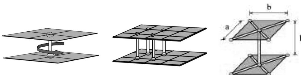
Figure 2 Standard nodal connection (left), multiple beam connection (center), single beam with torsional resistance by cross beams (right)
