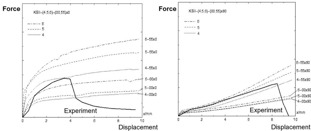
Figure 6 Measured spotweld forces vs. displacement for varied mesh density and varied location of the spotweld nodes for nodal connections; pure shear ( $0^\circ$ ) and pure tension ( $90^\circ$ )
