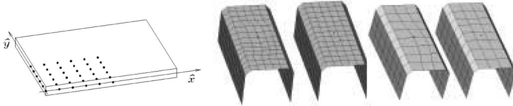
Figure 5 Variation of mesh density and location of connection nodes within elements
