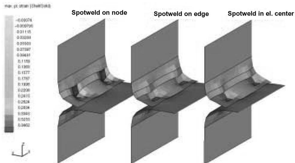
**Figure 13 Deformation pattern of multiple spotweld example under pure shear load-ing; continuum spotweld; partial view**
