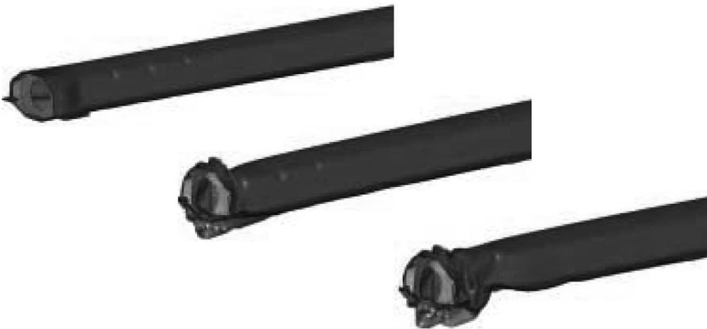
**Figure 15** Longitudinal girder model under crash loading; deformation states; contact shell set spotweld model
