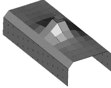
Figure 10 Deformation of specimen for connection via contact-shell-set; 0° (pure shear, side view) and 90° (pure tension, top view) loading. Location of contact shell set varied.
