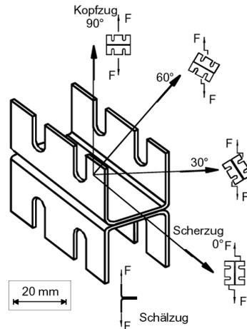
**Figure 1 Specimen for single spotweld investigations under varying loading direction**
