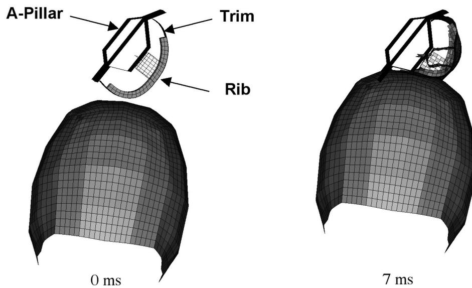
Figure 6: Head impact of A pillar
