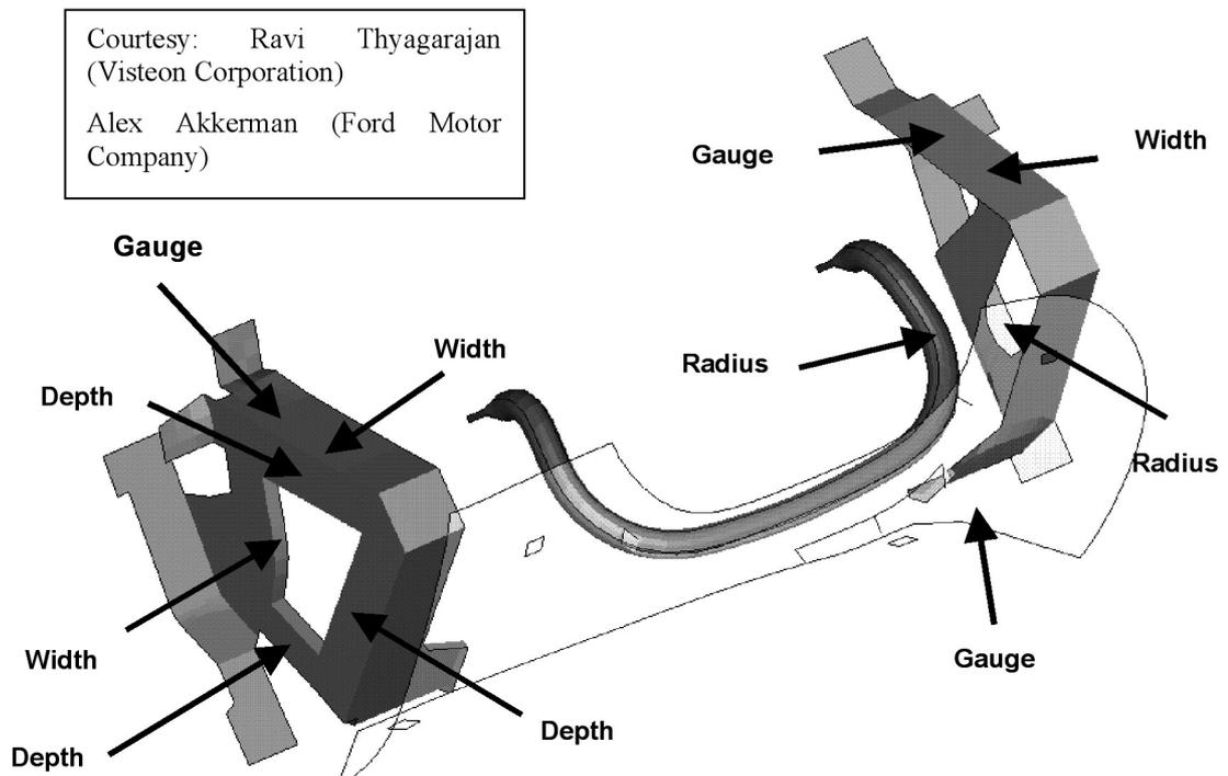
Figure 2: Design variables of the knee bolster system
