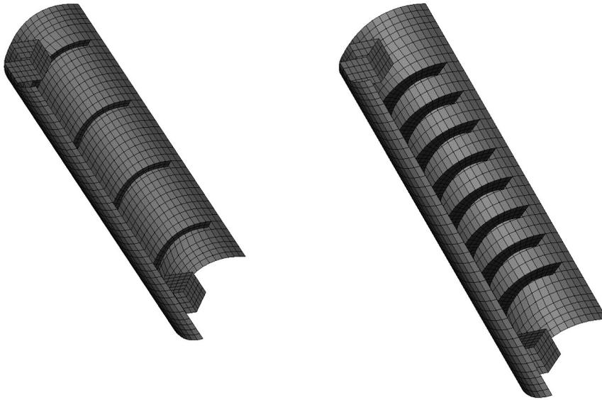
Figure 7: Baseline (left) and Optimal (right) designs
