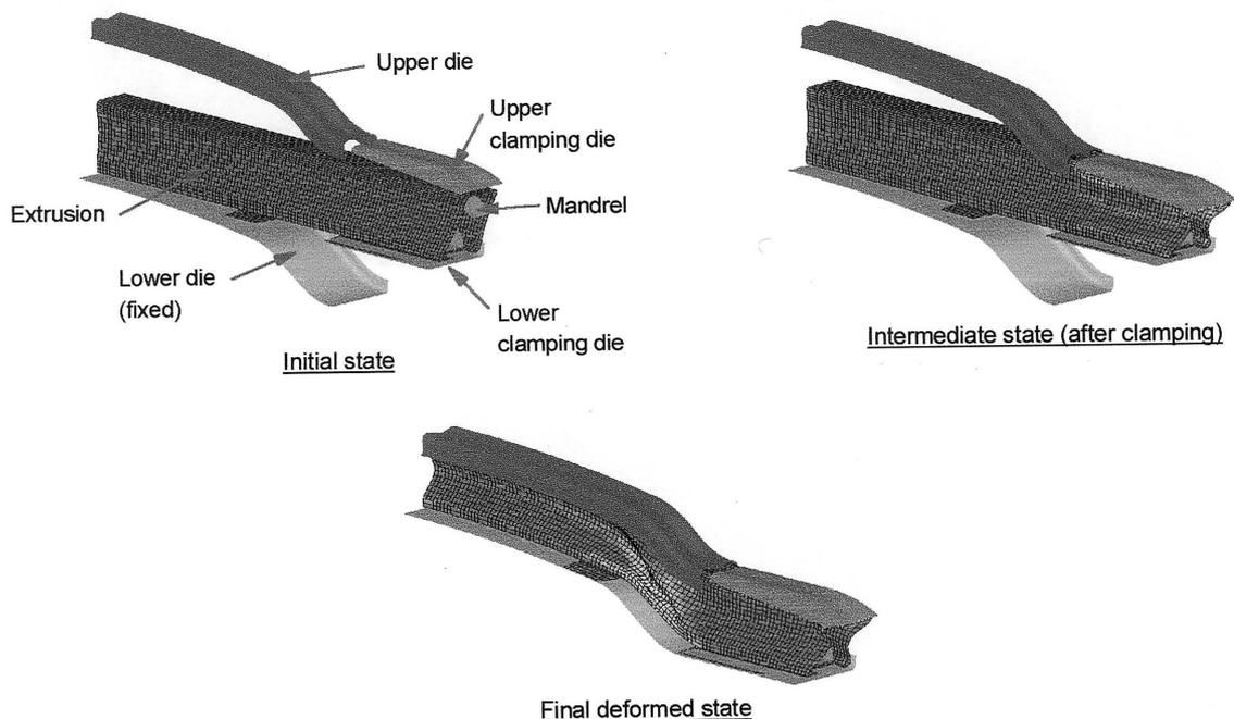
**Figure 3: The FE model shown at three different stages.**
