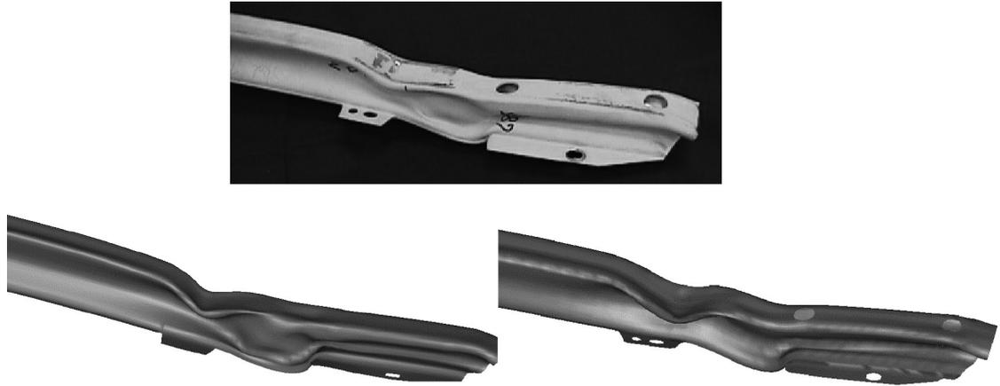
**Figure 10: Comparison of deformations after crash for the test (above), simulation based on Case I geometry (left) and nominal geometry (right).**
