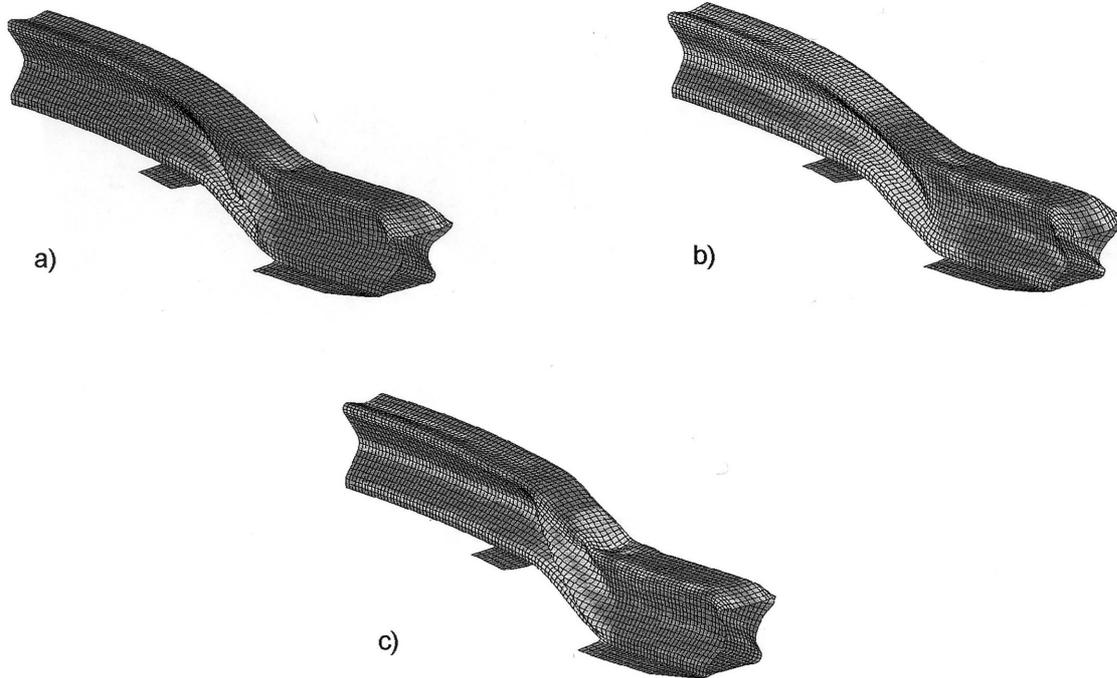
Figure 4: Deformed mesh (i.e. final geometry) for the three process alternatives investigated.
