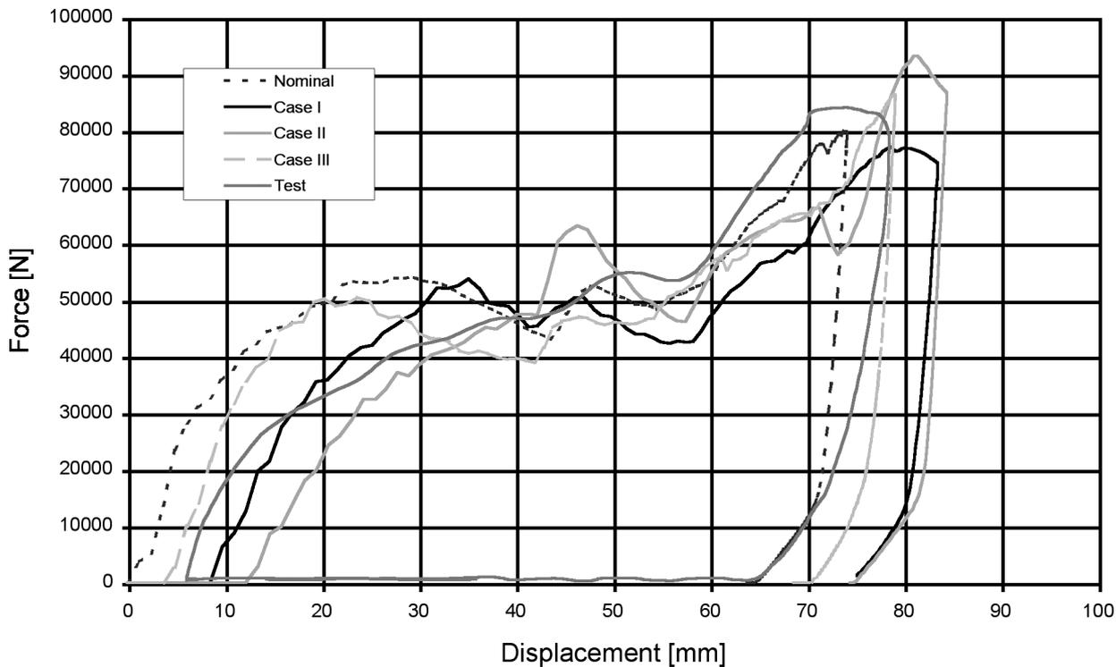
**Figure 9: Load-displacement curves obtained by simulations and testing.**
