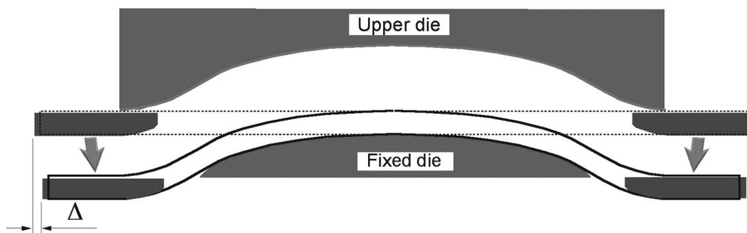
Figure 2: Schematic view of the forming process.
