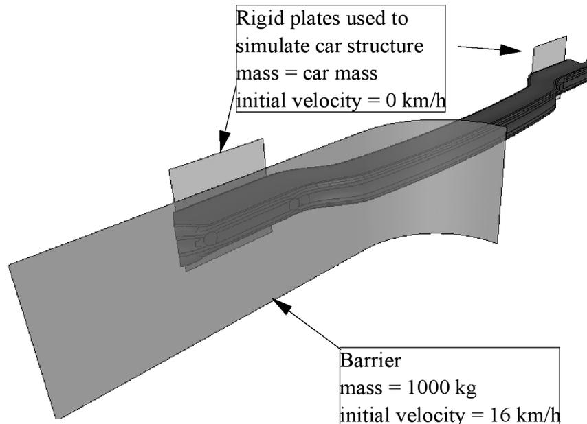
Figure 8: FE-model for crash simulations
