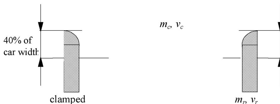
Figure 7: General set-up for the AZT 40% offset crash test.
