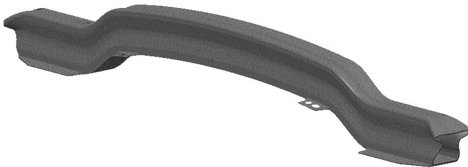
Figure 1: CAD model of the investigated bumper beam.
