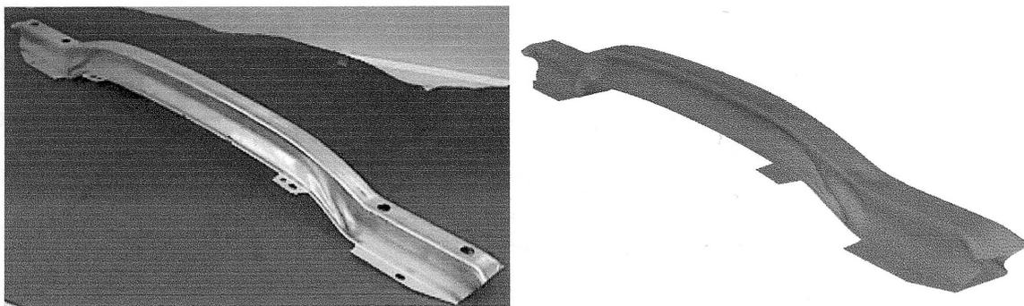
Figure 6: Comparison between real product and simulated geometry.
