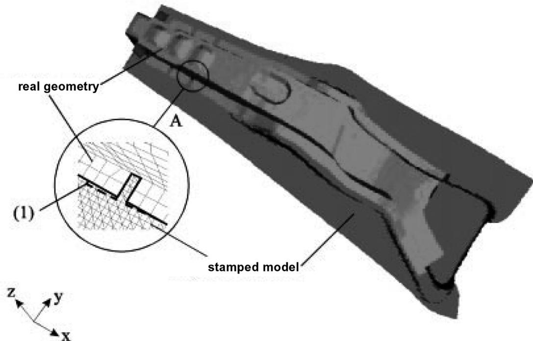
Fig. 7: Comparison of stamped panel and side rail design geometry
