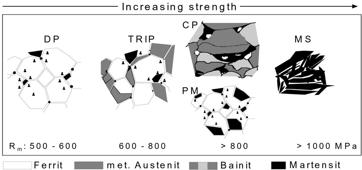
Fig.1: Metallurgical aspects of DP and TRIP steels [3]
