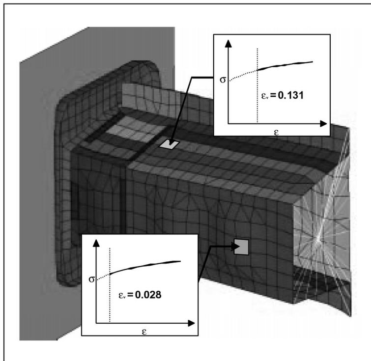
Fig. 9: Model of front rail considering the effects due to the stamping process
