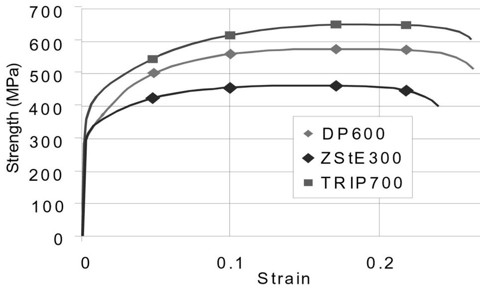
Fig. 2: Engineering stress-strain curves of DP600, TRIP700 and ZStE300 steel
