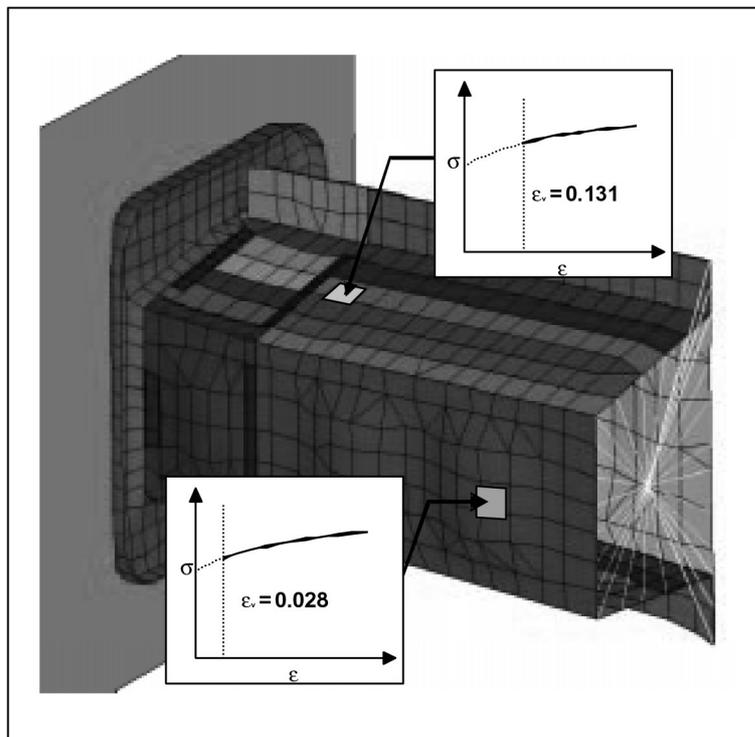
Fig. 9: Model of front rail considering the effects due to the stamping process
