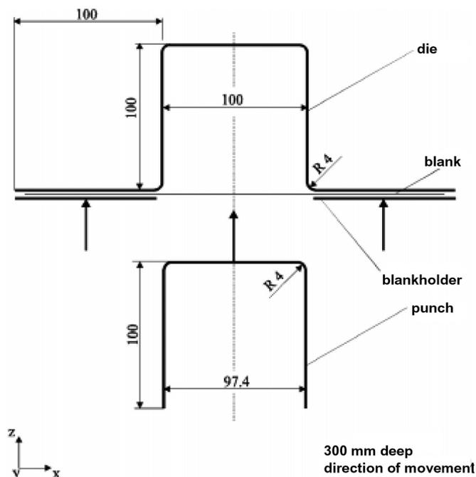
Fig. 5: Tool geometry for stamping simulation of an U-shaped profile
