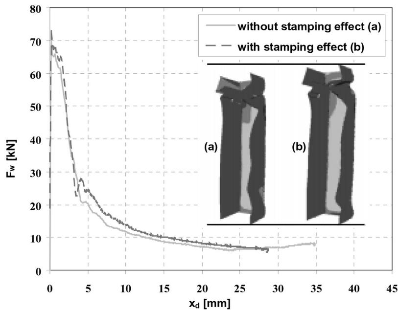
Fig. 6: Force-deflection curve with and without stamping effects - DP500
