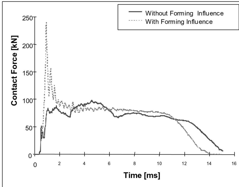
DP600  $t_0 = 1.66 \text{ mm}$   $V_0 = 15 \text{ km/h}$
