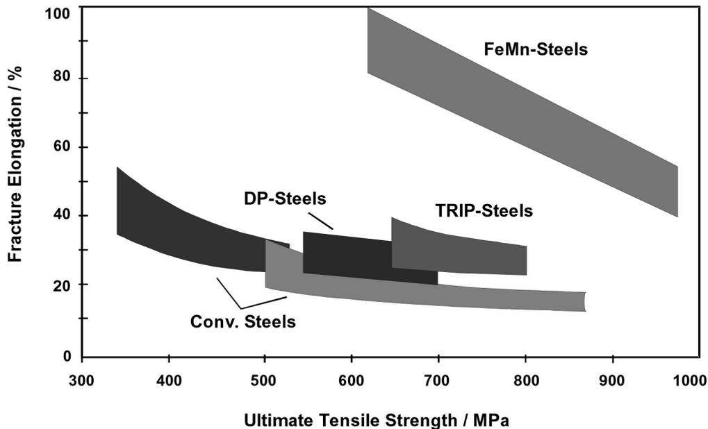
**Fig. 3: Fracture elongation versus ultimate tensile strength of different steels**
