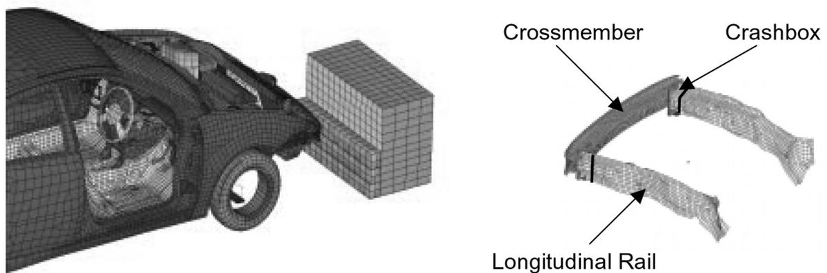
Fig. 4: Finite Element Model of a front end substructure with side rail
