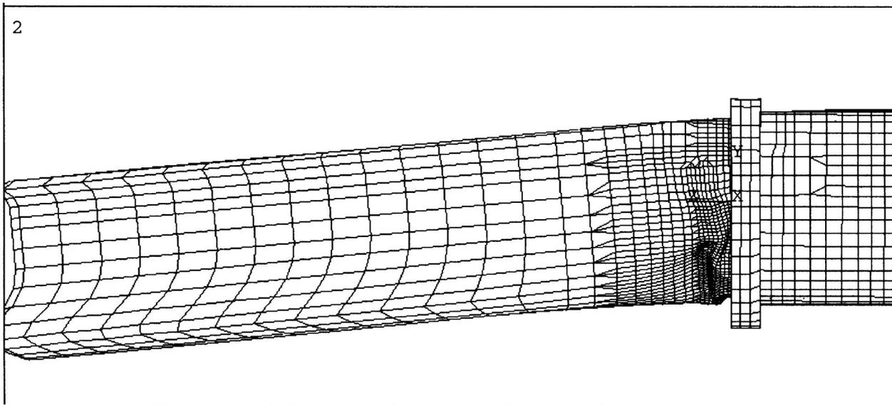
**Fig. 10: Buckling state with the original thickness distribution; real structure; transient analysis**
