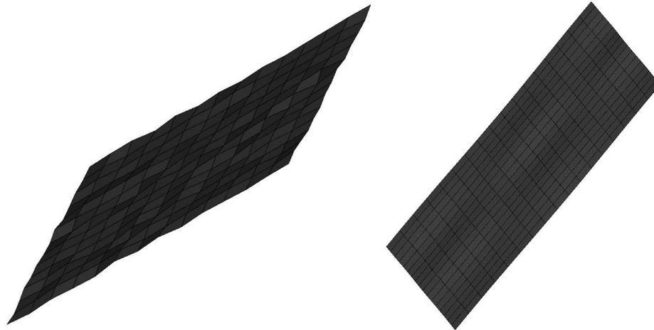
**Fig. 8: Random and sinusoidal distribution of imperfections**
