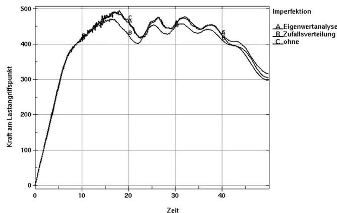
**Fig. 9: System response for different types of imperfections:
