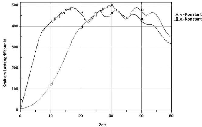
**Fig. 4: Load-versus-time curve for A) constant velocity and B) constant acceleration**
