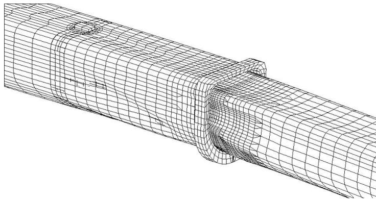
**Fig. 11: Buckling state with a slightly modified thickness distribution; real structure; transient analysis**
