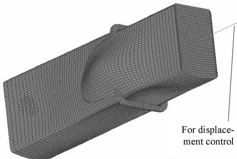
**Fig. 7: First buckling mode of telescope arm; simplified model**
