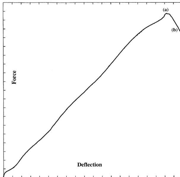
**Fig. 2: Load-deflection diagram of the telescope arm of a crane, real system**
