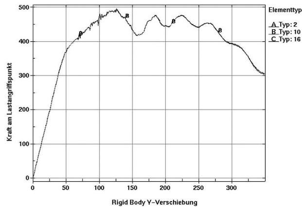
**Fig. 3: Load-deflection curve for the telescope crane; model problem; transient analysis**
