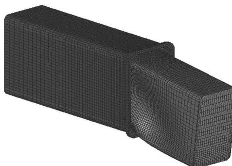
**Fig. 1: Simplified model of part of a telescope crane at the onset of buckling**
