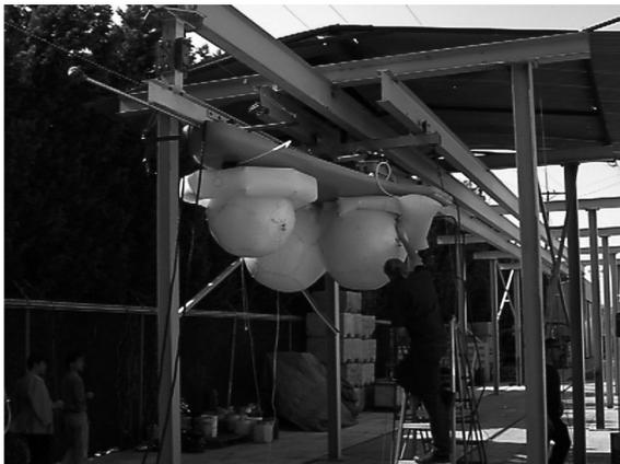
**Figure 5 – Airbag Drop Test Facility
