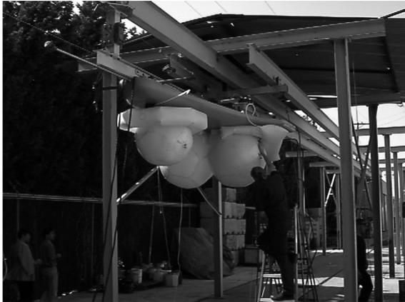
**Figure 5 – Airbag Drop Test Facility
