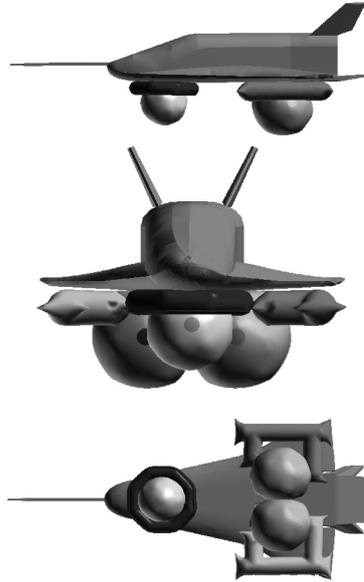
**Figure 2 – Final Airbag Configurations**
