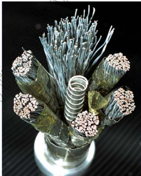
Figure 1: ITER Toroidal Field Model Coil TFMC Nb 3 Sn superconducting cable, courtesy of ENEA-FRASCATI
