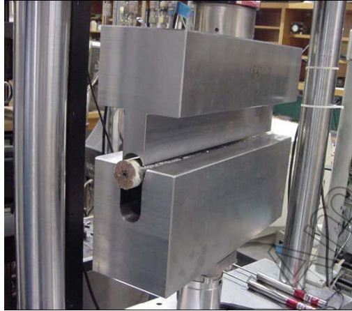
Figure 10: An NHMFL transverse pressure apparatus for mechanical characterization of a variety of ITER-relevant cable designs for the US ITER Magnet Team
