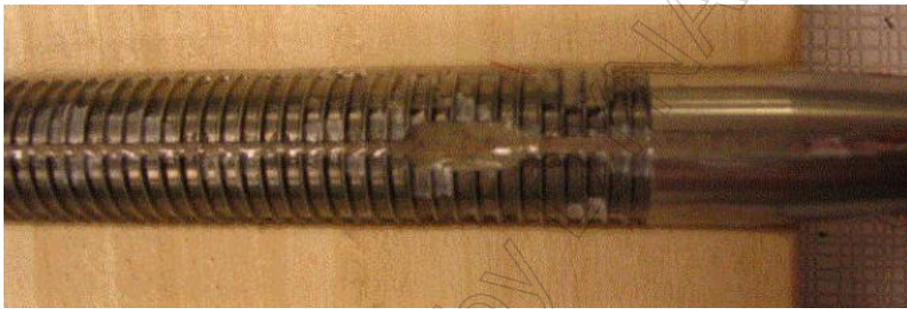
Figure 10: Instrumented ammunition. Strain gauge implemented on the rod (left), complete round with flare (right)
