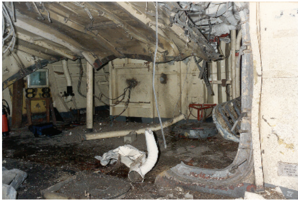
Figure 1 Roofdier Trials internal explosion
